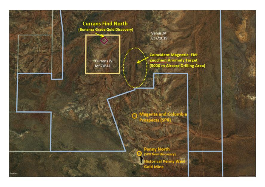
Figure 1. Location of 5000m Aircore drilling along the Penny West Shear (coincident magnetic-EM-geochem anomaly target)
