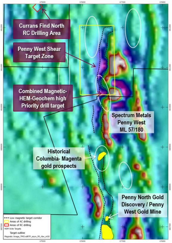
Figure 2. Area of Aircore Drilling along the Penny West Shear shown on regional aero-magnetic anomaly map
