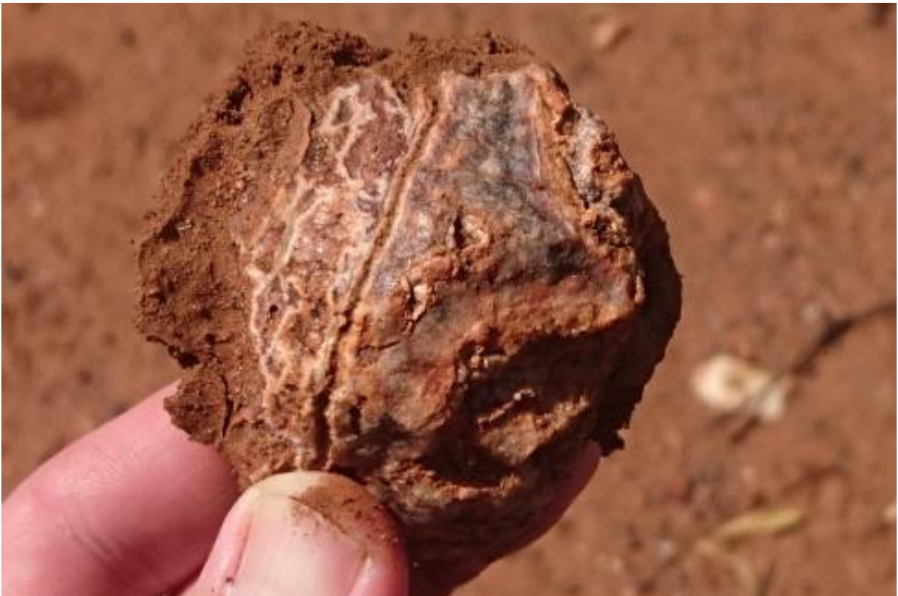
Figure 11: Epithermal vein float on Nepean tenement M15/709 with breccia fragments rimmed by colloform quartz
