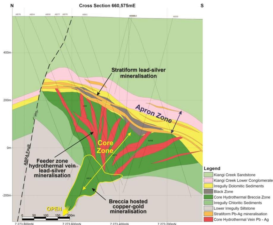
**Figure 5: Stylised geological cross section of Abra at 660,575mE looking east**
