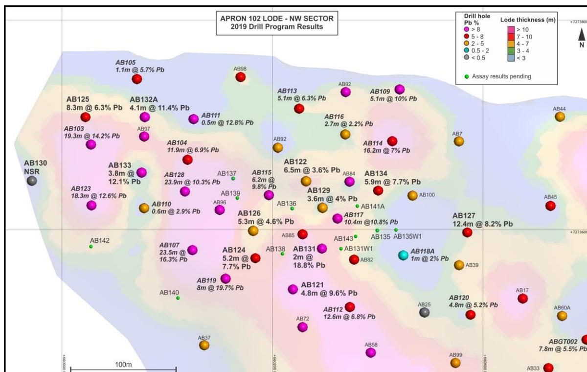
**Figure 3: Plan view of the Apron 102 Lode showing drillhole pierce points (coloured by lead grade) and lode thickness contours**
