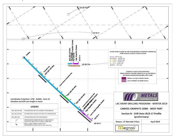
Figure 3: Drill hole plan view section of LR19-17 at the Lac Rainy Graphite Project
