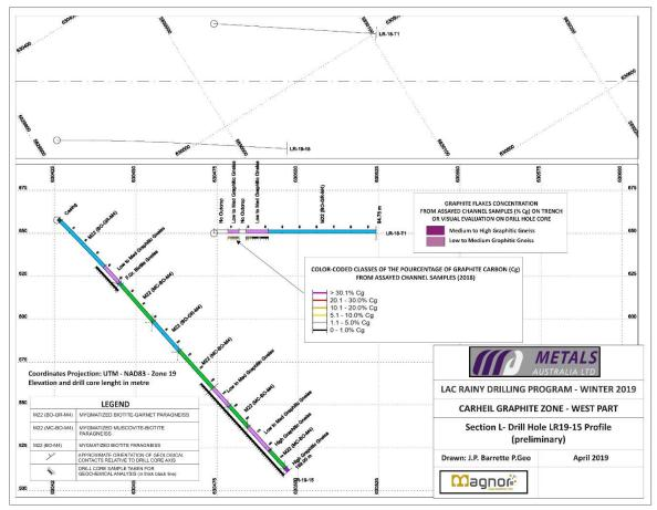
Figure 4: Drill hole plan view section of LR19-15 at the Lac Rainy Graphite Project
