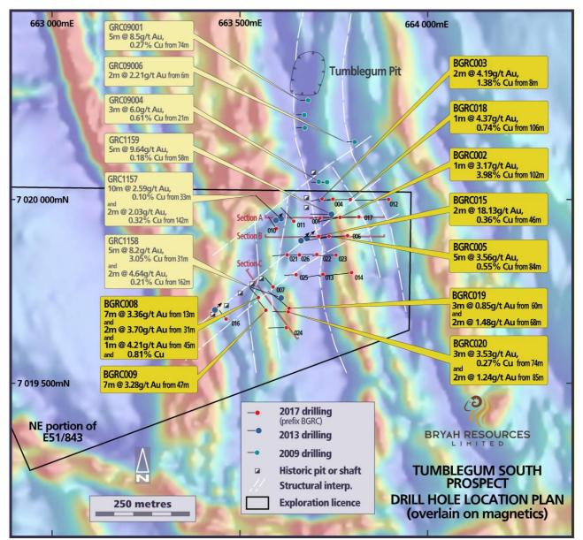
Figure 2 – Drill Hole Location Plan
