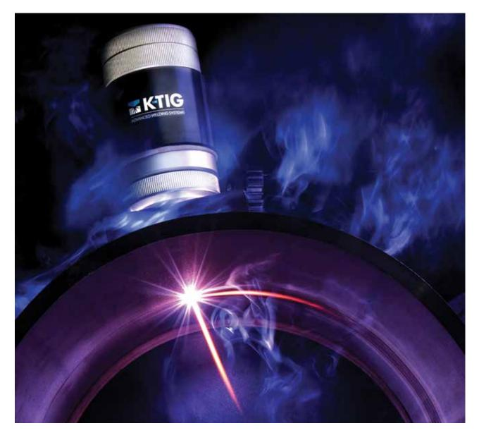
The K-TIG System combines the high-quality and cleanliness of GTAW with a depth of penetration that exceeds that of conventional gas-tungsten arc, gas metal arc and plasma welding processes.
