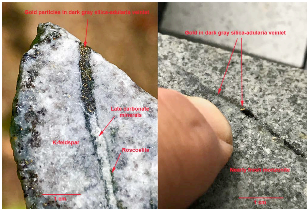
Figure 2: High-grade gold veinlets typical of the main gold mineralizing stage at in the Navilawa Caldera. Virtually all significant gold intervals examined in core exhibit narrow dark grey silica-adularia veinlets, occasionally with fine specks of native gold. Their dark gray color comes from fine pyrite or other minerals, perhaps tellurides, scattered throughout the silica-adularia. Dark green roscoelite often occurs along their margin. Late, white to tan carbonate minerals are sometimes present, usually filling voids within veinlets. Very subtle K-feldspar alteration appears to penetrate surrounding wallrock over a few millimeters to centimeters. Traces of disseminated pyrite are sometimes present in wallrock alteration.
