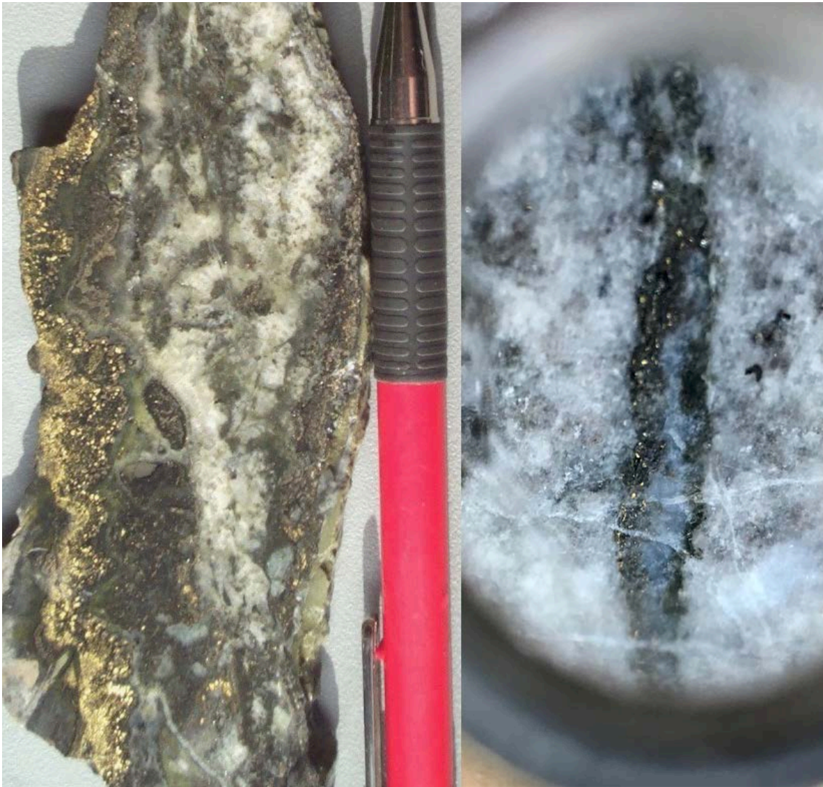
Figure 3: A 3 cm-wide high-grade gold vein from Porgera (left) and a 1.5 mm-wide high-grade gold veinlet from Navilawa (right). Gold in the sample from Porgera (along the left side of the sample) is intergrown with fine dark gray silica-adularia. Roscoelite (green) forms patches throughout the sample and carbonates (white) are late and occupy the core of the vein. The veinlet from Navilawa displays remarkably similar mineralogy and style to the vein from Porgera. Gold is intergrown with dark grey silica-adularia along the left margin of the veinlet. Dark green roscoelite is visible along the right side of the veinlet, and white carbonates fill the core. Dr. Hennigh believes this comparison is critical to demonstrating the gold system at Navilawa is indeed of the same alkaline type. Moreover, it is entirely possible that more robust versions of the veinlet seen on the right have yet to be discovered at Navilawa.
