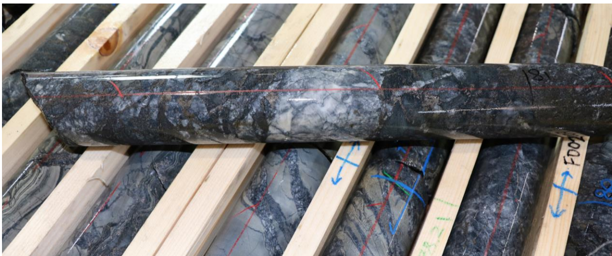
Figure 9. Quartz-carbonate-sulphide veined breccia, with quartz-carbonate-sulphide veined albitites in background from FAKD0006.
