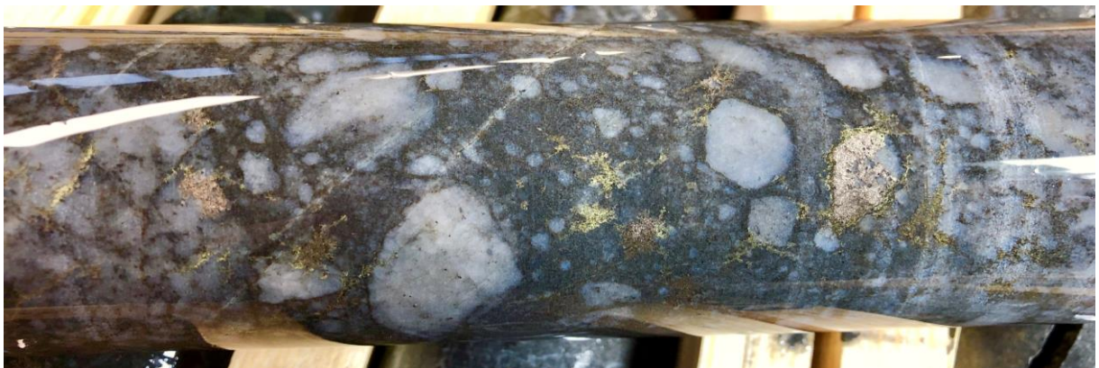
Figure 6. Milled breccia with variable sized rounded clasts of quartz and stringers of chalcopyrite and pyrrhotite from FAKD0003.
