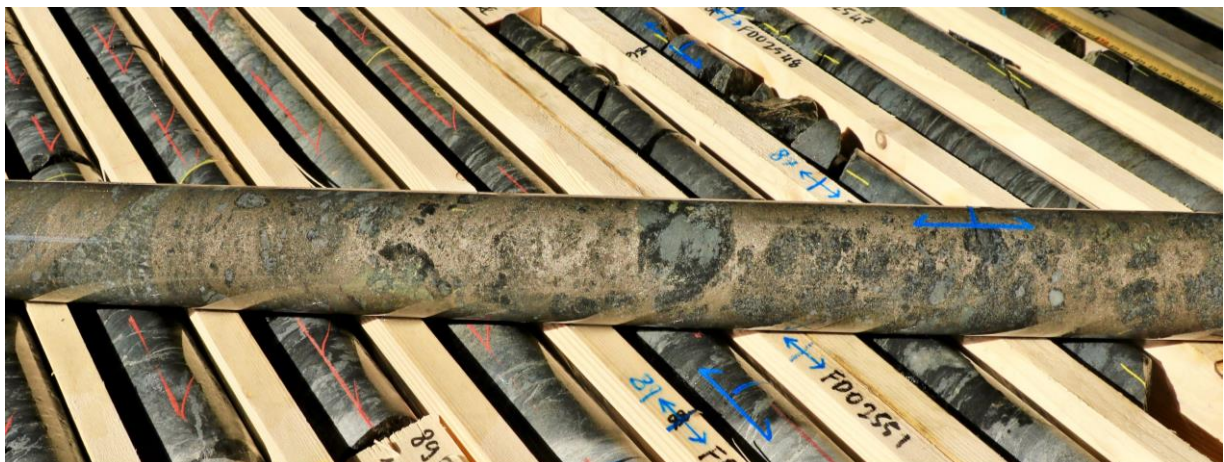
Figure 3. Semi-massive and breccia sulphide (mainly pyrrhotite) from FAKD0003.
