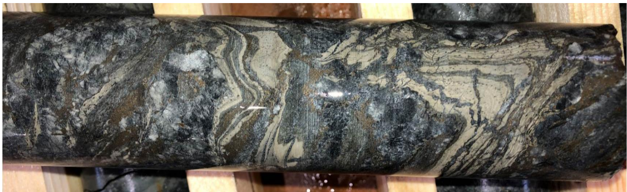
Figure 8. Folded, veined and brecciated albitite in FAKD0004.
