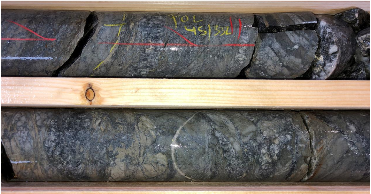
Figure 7. Multiple generations of albitisation, veining, and brecciation in FAKD0004.
