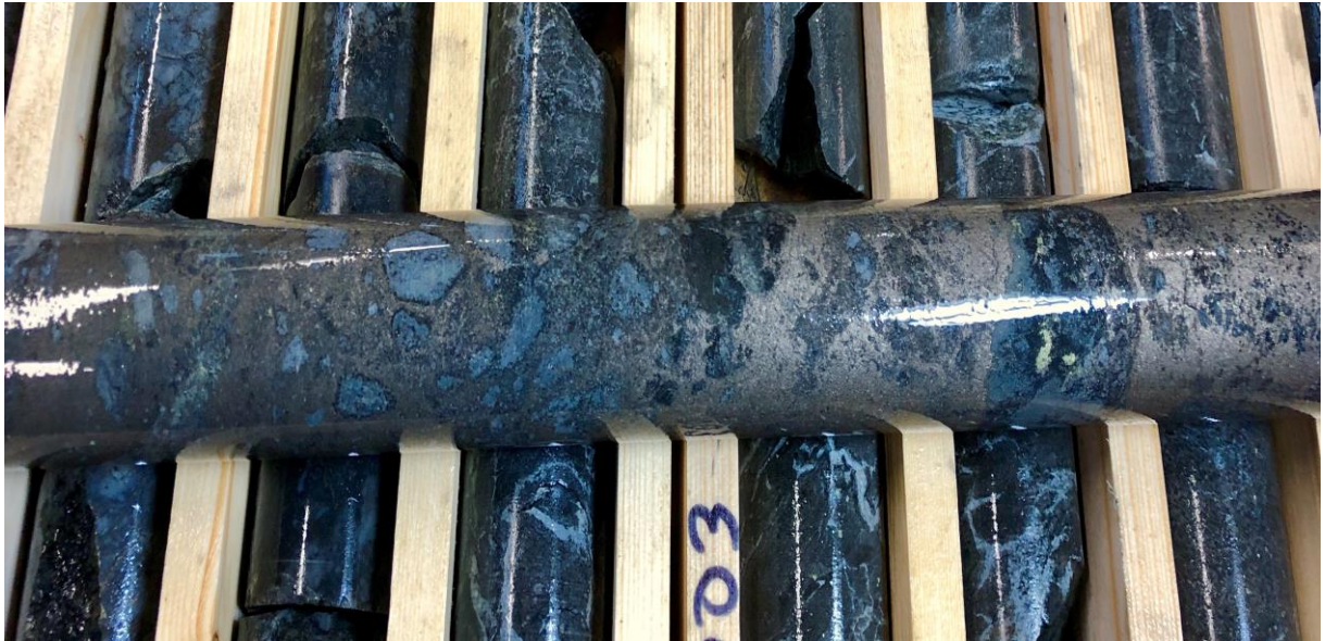
Figure 4. Milled breccia with quartz and wallrock clasts in a sulphide matrix from FAKD0003.
