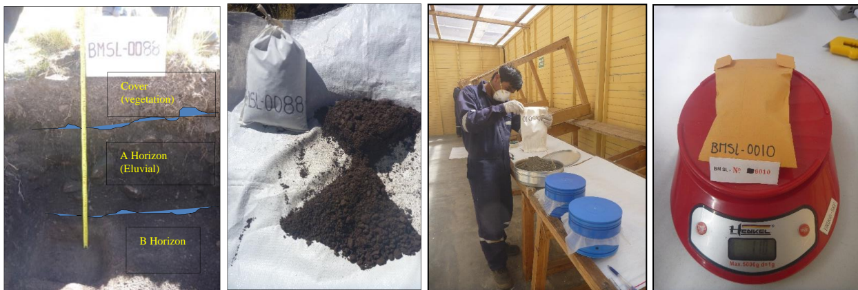
Figure 8 ABOVE : Example of the soil sample procedure, left to right: sampling at a prescribed grid location, retention of a soil sample, in-camp sieving (after it's dried), bagging and labelling for submission for geochemical analysis.
