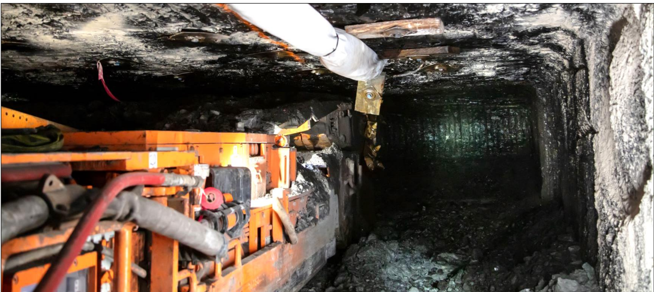
Figure 1: CM at Poplar Grove making a ~20 ft cut into the Western Kentucky No.9 coal seam
