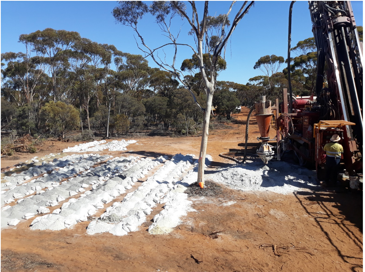
Photo 1: Drill cuttings from PDRC263. White coloured piles are pegmatite. 136m of pegmatite was intersected in this hole.
