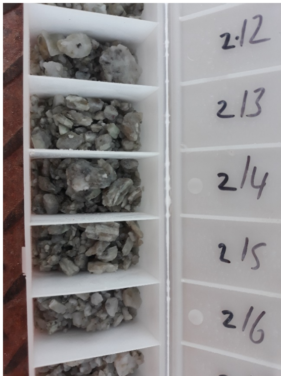
Photographs 2 and 3: Examples of washed drill cuttings from PDRC263. In each cell one of the pale minerals identified through visual appraisal by Company geologists, with confirmation determination by Raman spectrometry, is spodumene.
