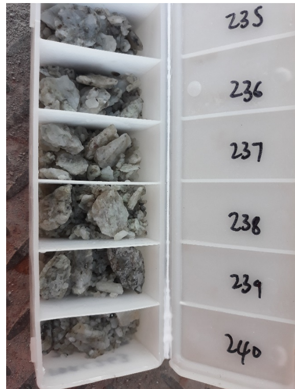
Photographs 2 and 3: Examples of washed drill cuttings from PDRC263. In each cell one of the pale minerals identified through visual appraisal by Company geologists, with confirmation determination by Raman spectrometry, is spodumene.
