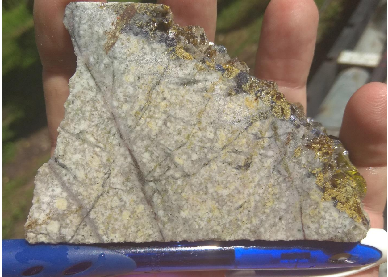
GDD042 113.30m Crackle fractured silica-sericite altered diorite porphyry with early quartz veins crosscut by later stage sulphide-rich fractures and veins. Prominent yellow sphalerite-galena open space vein fill (interval assay 1m @ 8.04g/t au, 7.3g/t Ag)
