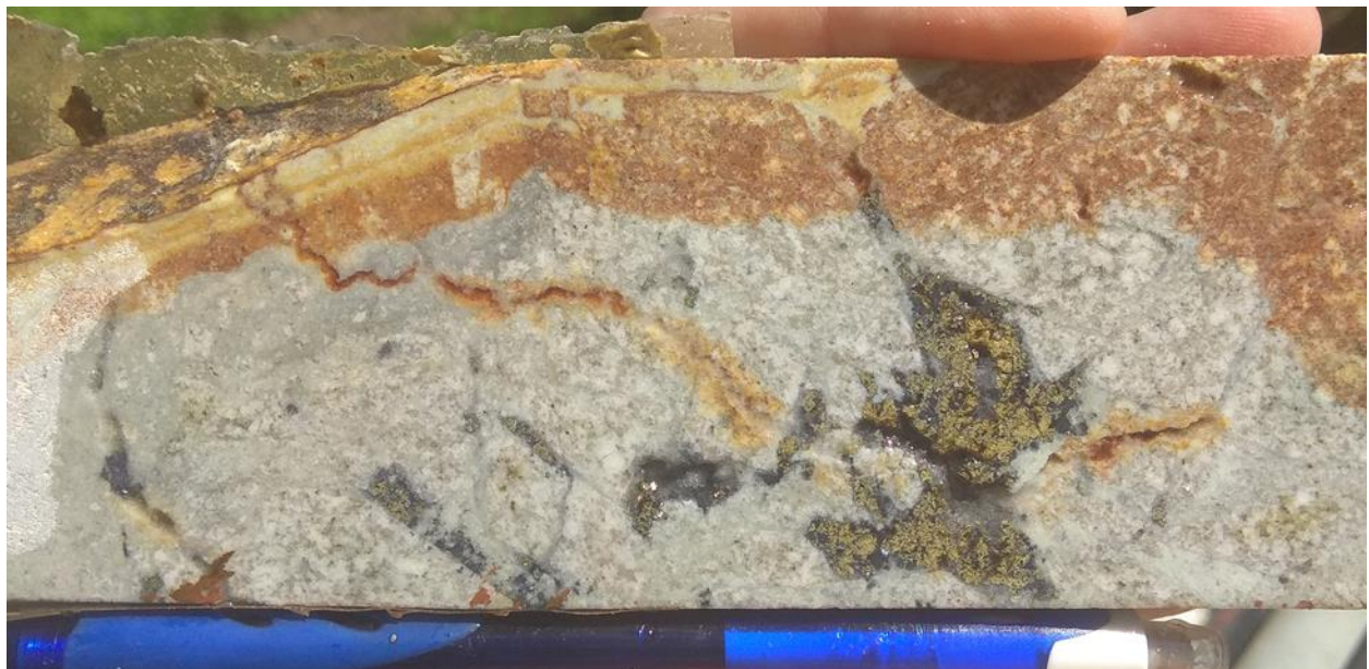
GDD042 43.30m Crackle brecciation with quartz-sphalerite-galena infill in silica-sericite altered diorite porphyry (interval assay 0.8m @ 8.19g/t au, 10.0g/t Ag)
