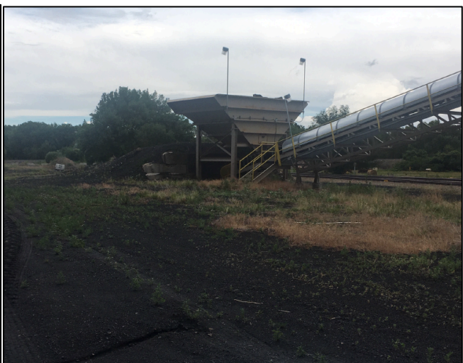
Image: feeding system into the rail loadout
