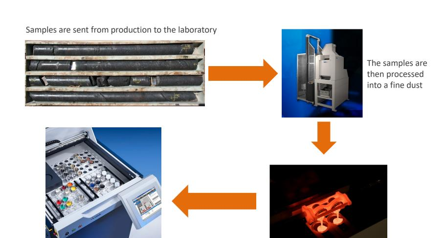
The glass disk is presented into an x-ray spectrometer for analysis
