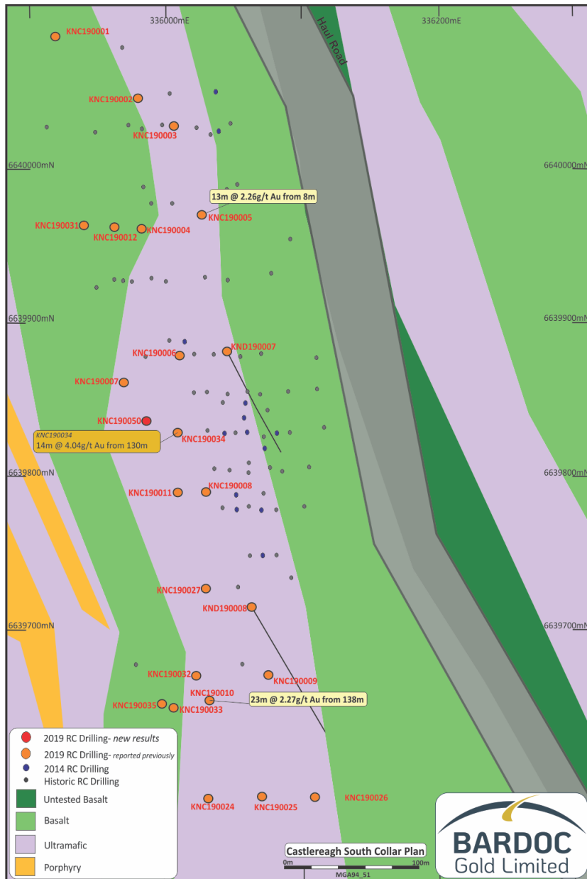
Figure 5. South Castlereagh drill-hole location plan
