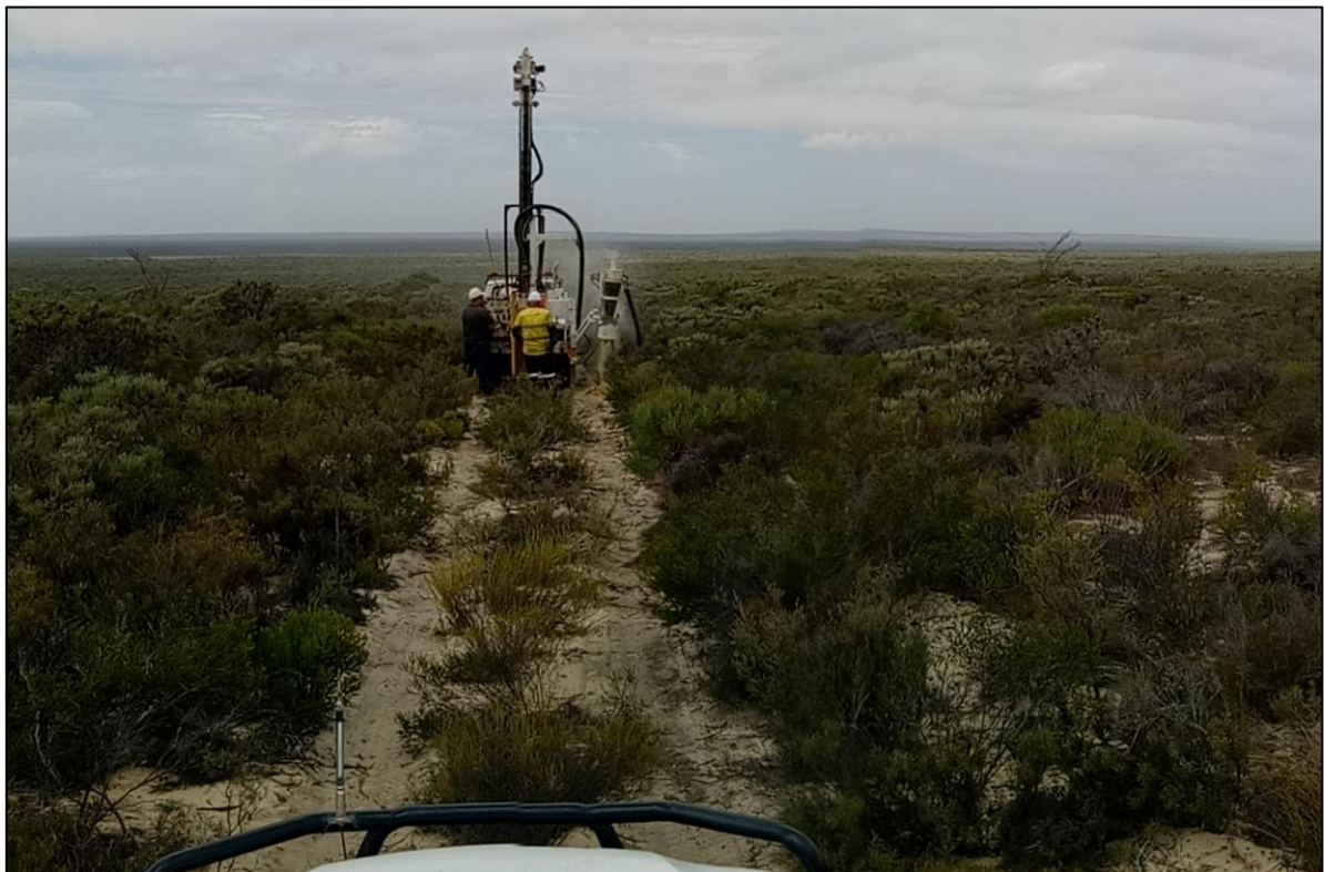
Figure 4: Landcruiser mounted Mantis 82 NQ sized aircore drill rig
