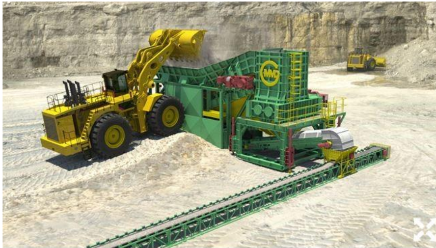
Figure 22: Mining process – silica sand loaded and screened
