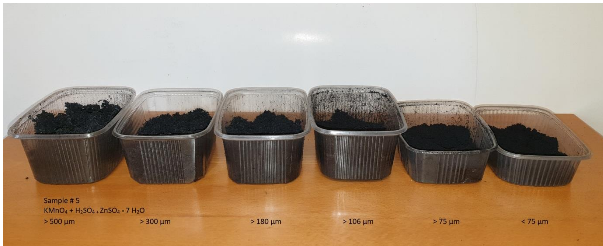
Figure 16 - Photos of BEM product from NGS following expandability test work
