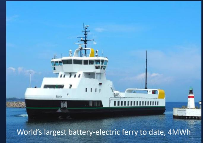
World's largest battery-electric ferry to date, 4MWh
