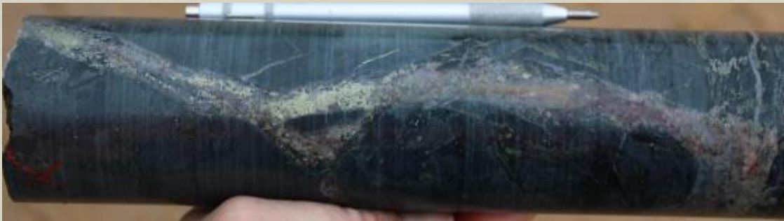
Anhydrite-magnetite-chalcopyrite veining in sediments at 594.9m.
