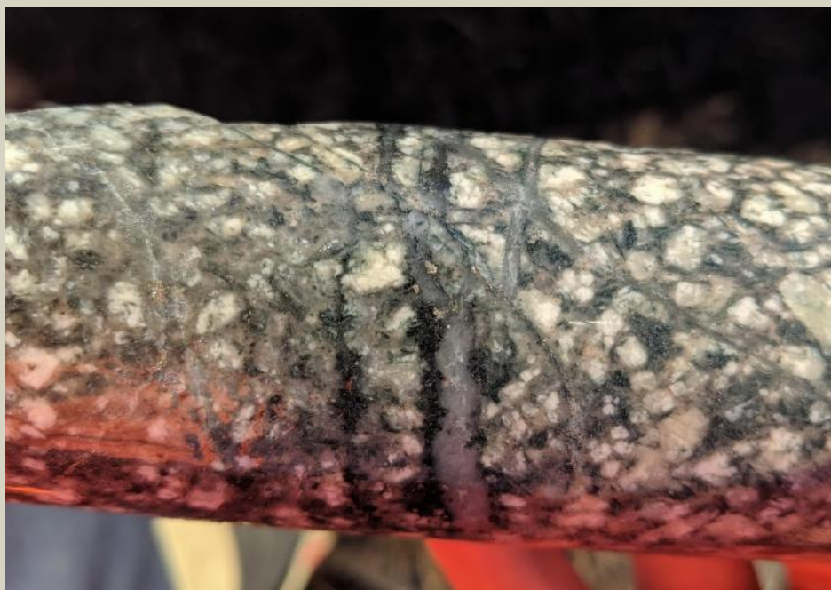
Quartz magnetite actinolite vein with pyrite and minor chalcopyrite in an actinolite albite pink altered QDP at 1667.2m
