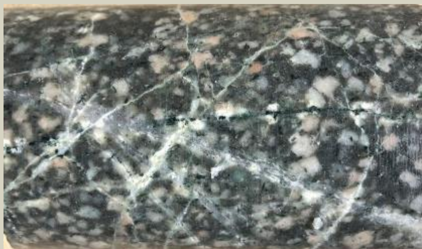
Probable actinolite vein cut by quartz A vein in QDP. 406.6m
