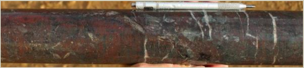
Specular hematite-chalcopyrite-magnetite-red hematite in sediments at 633.0m
