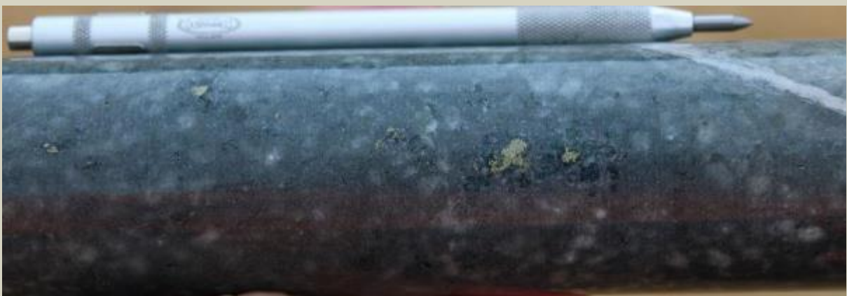
Chalcopyrite replacing some mafic sites at 1265.3m
