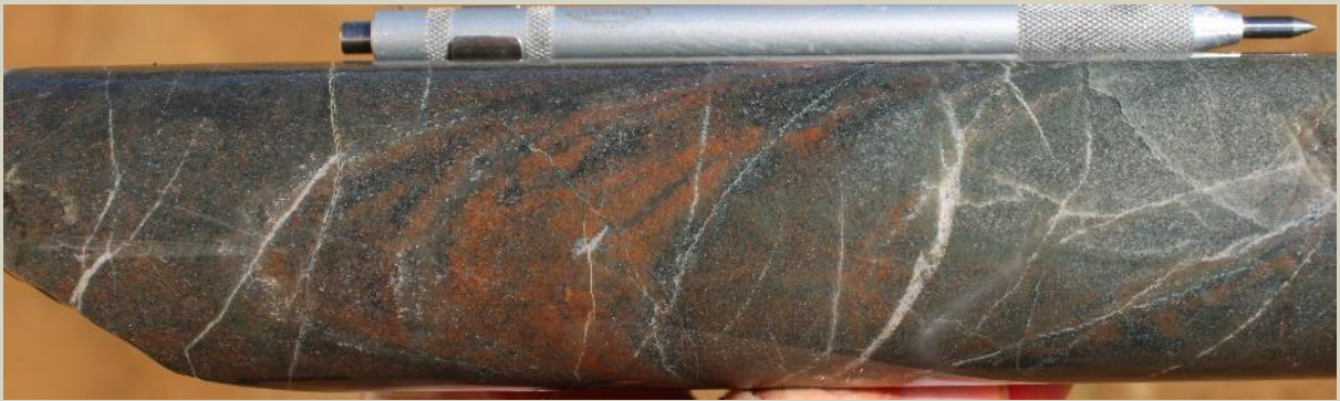
Hematite alteration halo to quartz veining in a sandstone at 1487.9m.
