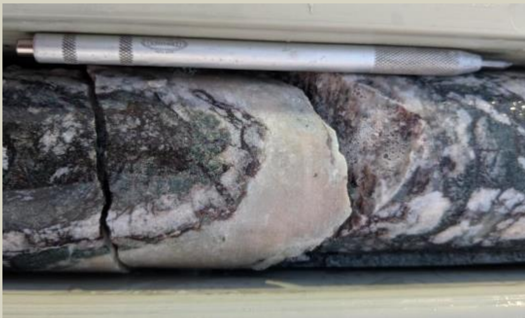
Anhydrite hematite vein at 1011.8m
