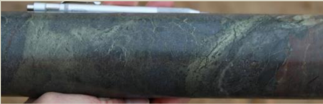
Chalcopyrite veining in sediments at 592.4m.
