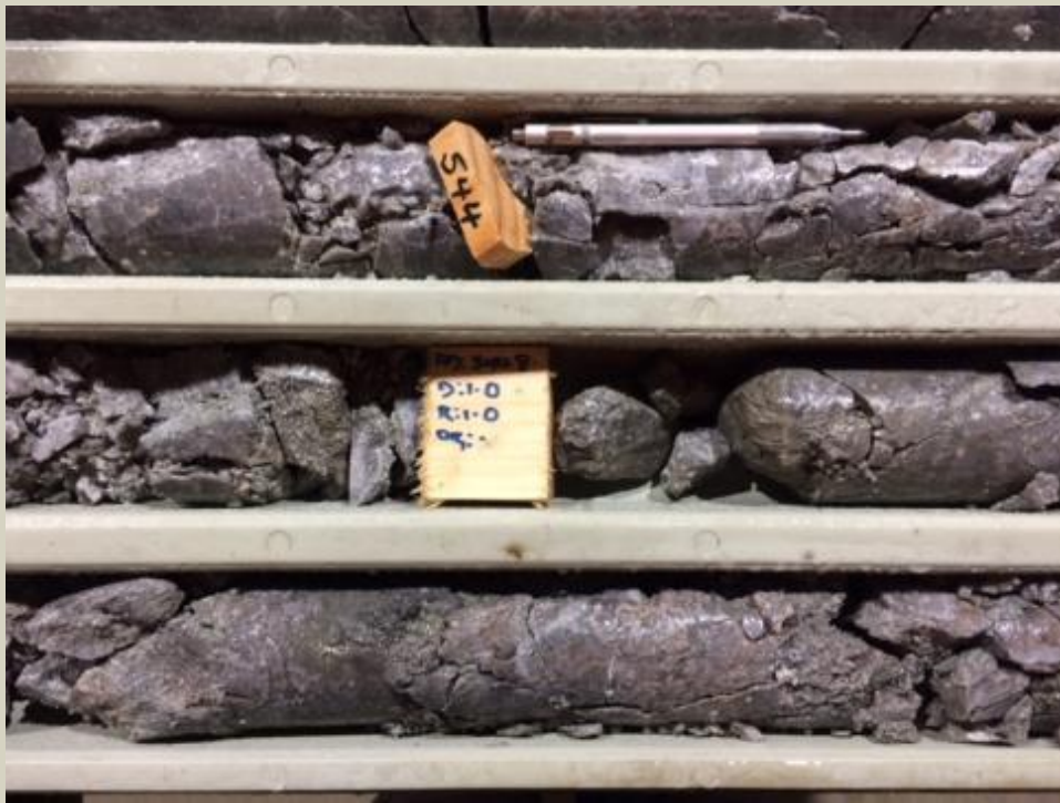
Sericite altered QDP with massive pyrite veining in a fault zone at 544m.
