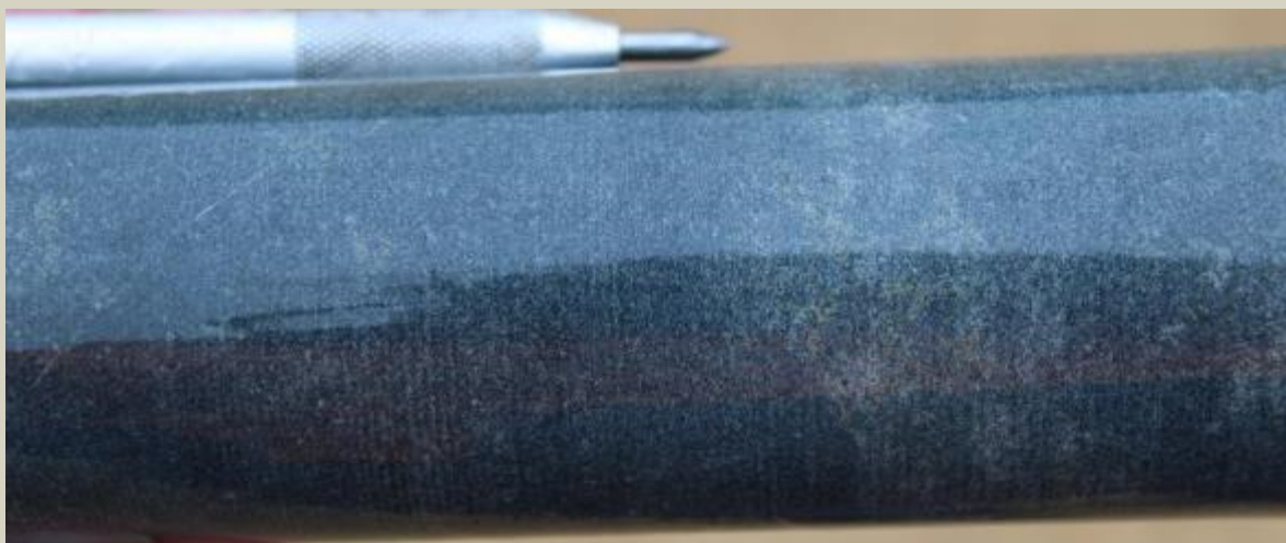
Epidote-pyrite+chalcopyrite in a sandstone at 1196.1m.
