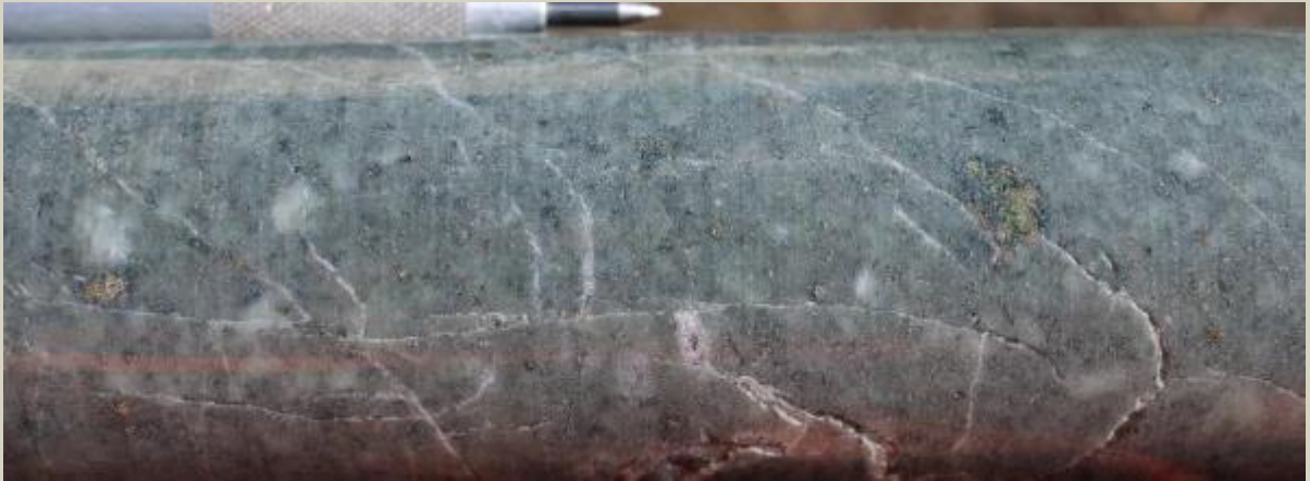
Quartz diorite porphyry with trace epidote-pyrite alteration at 1247m.
