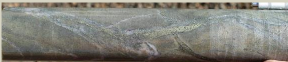
Anhydrite-chalcopyrite vein at 1234.2m.
