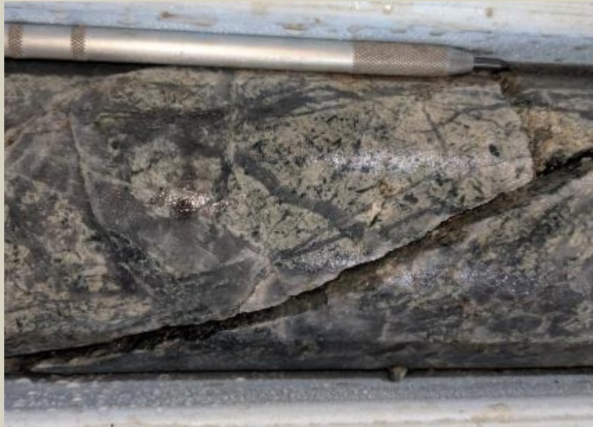
Well-developed M veining in QDP at 126m.
