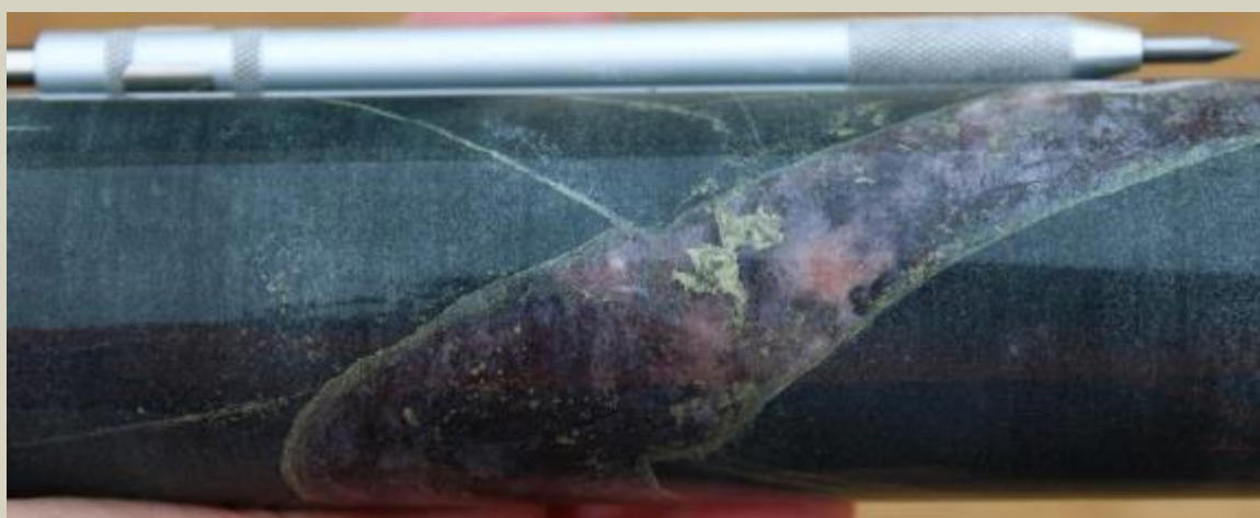
Anhydrite-magnetite-chalcopyrite-pyrite-epidote vein in sandstone at 1200.3m.
