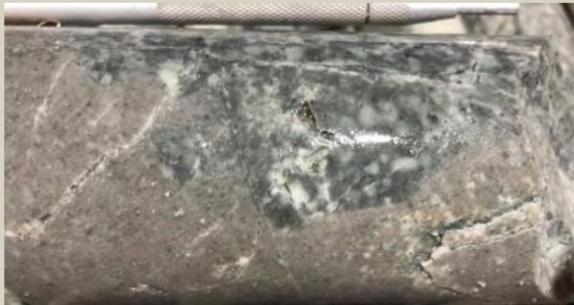
Contact between QDP (top) and finer grained quartz phyric diorite. 414.7m
