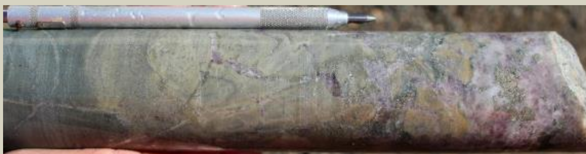
Anhydrite-pyrite veining in siltstone at 1221.9m
