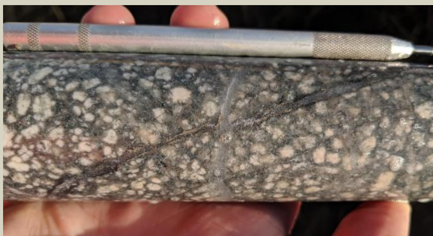
Railroad M vein with pyrite on margin, crosscut by quartz A vein at 1683m.
