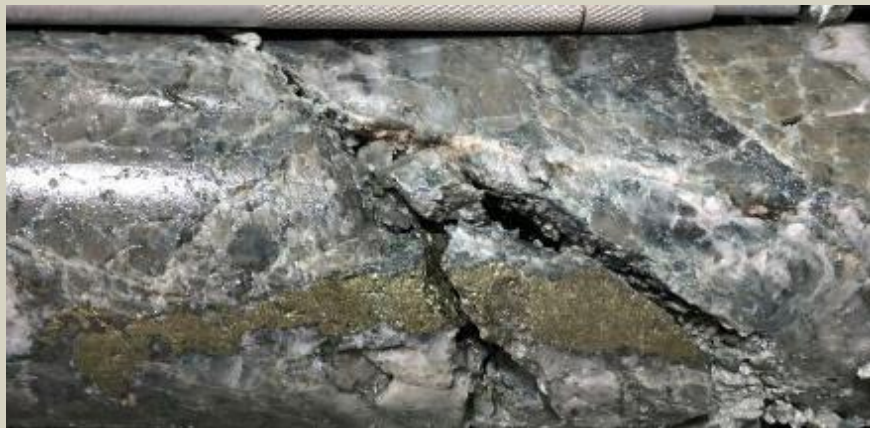
Chalcopyrite vein in QDP. 426.3m
