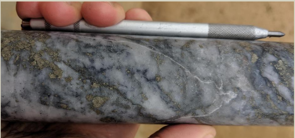
40cm wide quartz pyrite molybdenite vein at 1702.4m.
