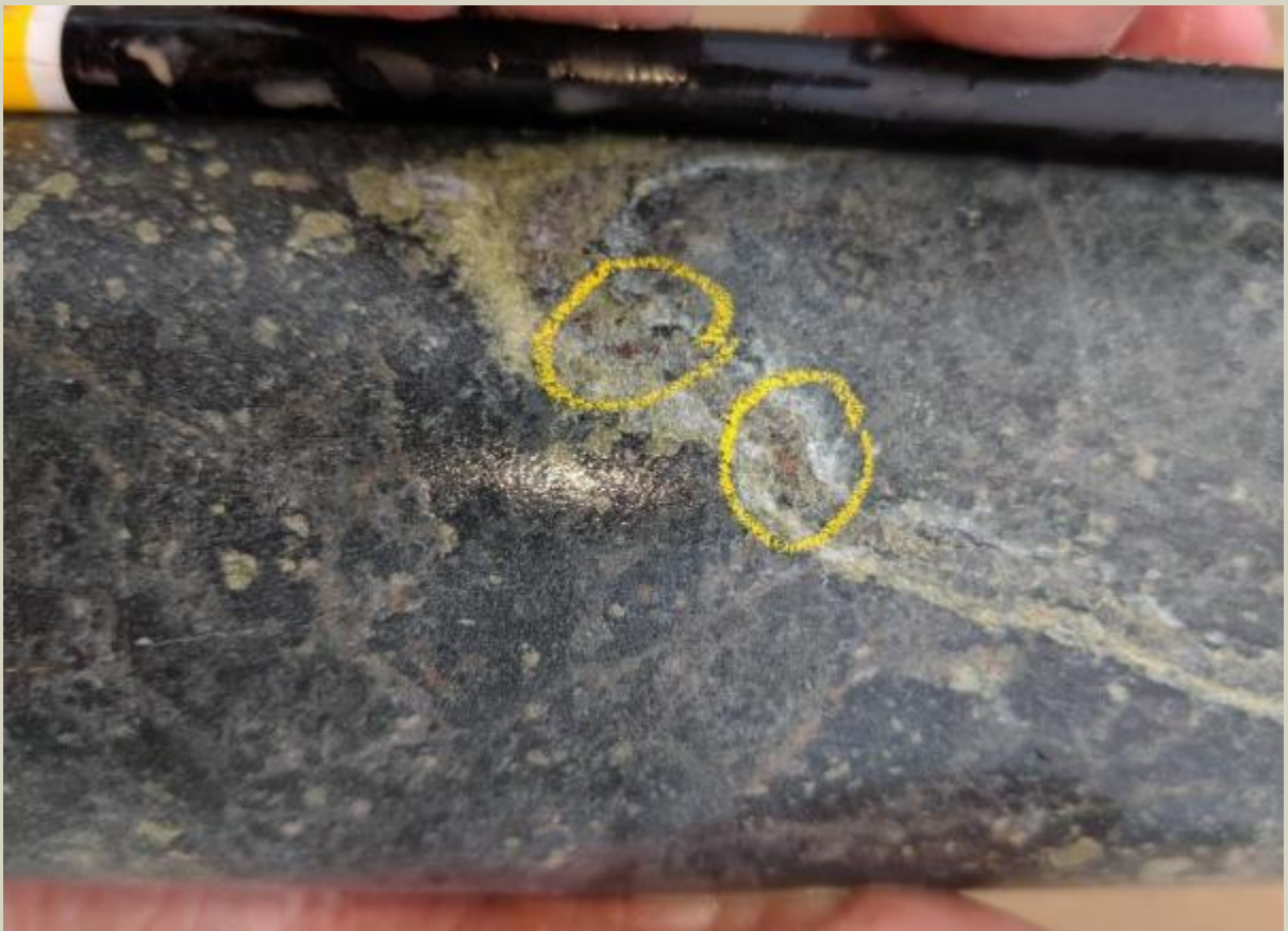
Trace quartz epidote bornite vein at 932.7mm
