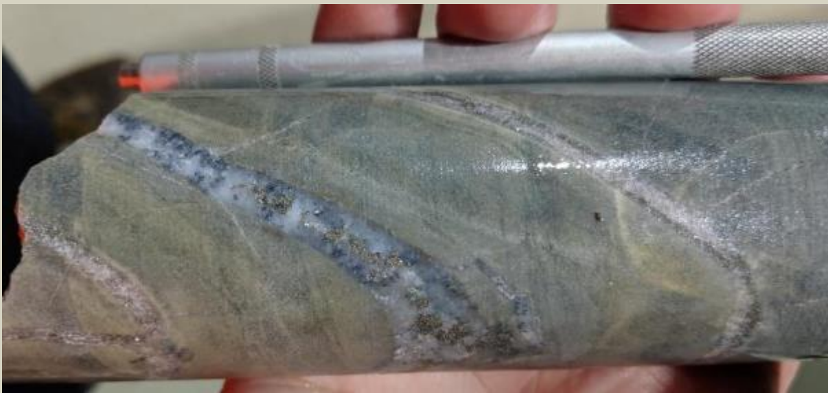
Quartz molybdenite pyrite A vein at 1339.6m
