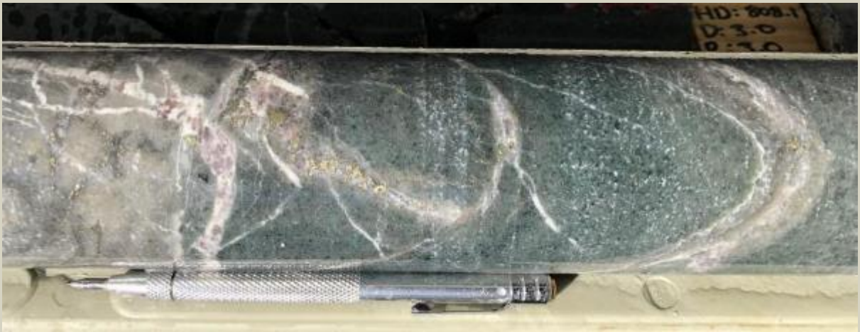
Anhydrite veins with chalcopyrite overgrowing earlier pyrite from 801m.
