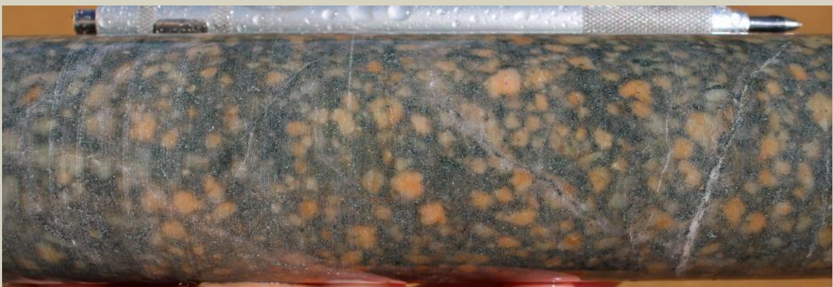
Quartz diorite porphyry with pinking of feldspar phenocrysts at 1467.8m
