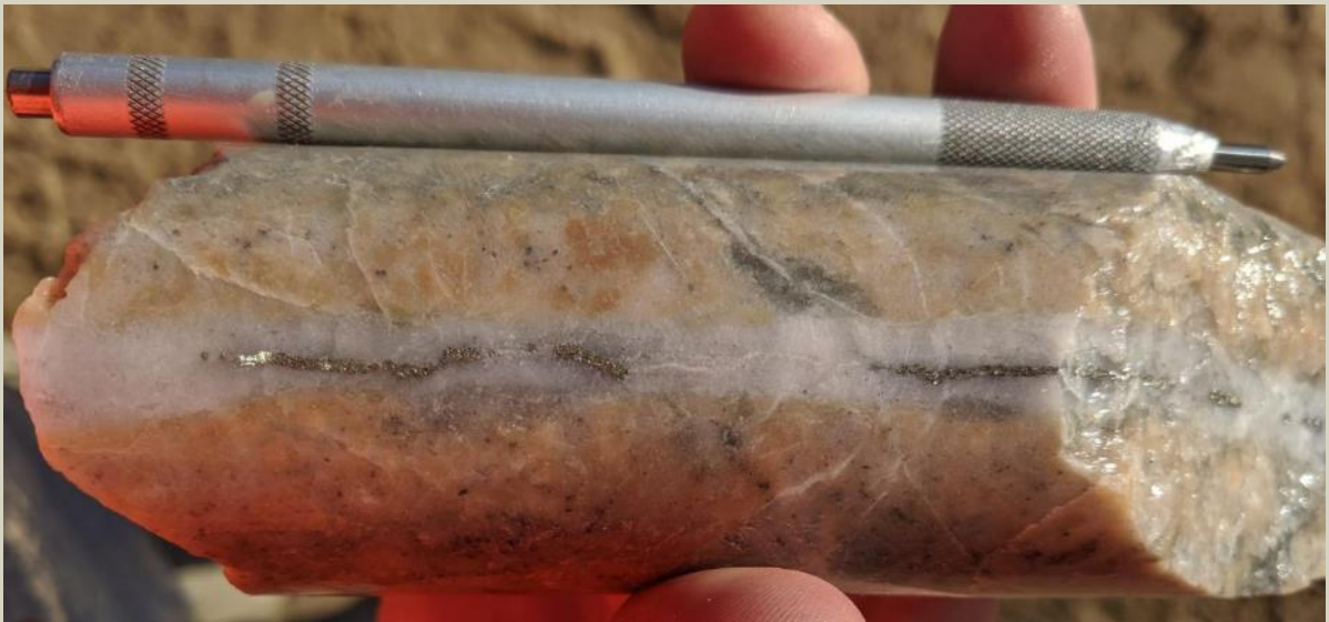
B vein with pyrite centre seam and sericite/ankerite? selvage at 1610.8m.
