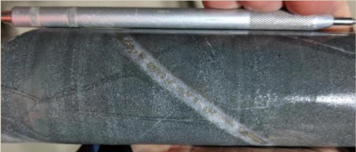
Quartz pyrite chalcopyrite A vein with centre seam 1333.6m.
