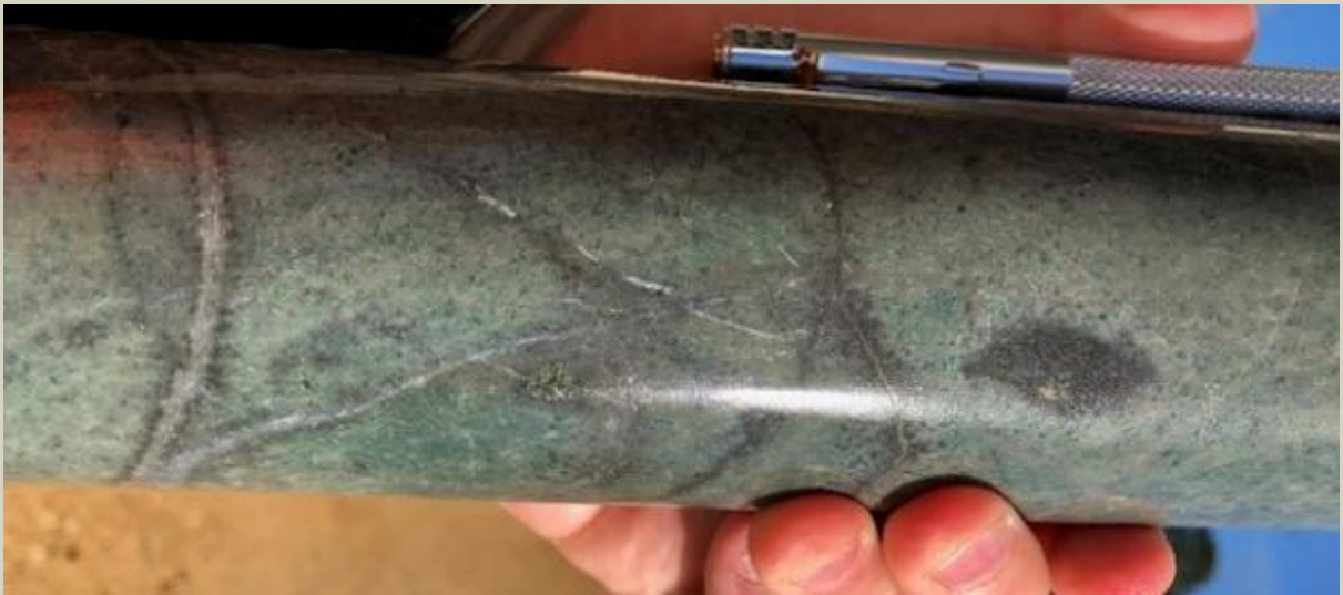
Biotite selvages to late veins and fractures with pyrite / trace chalcopyrite fill. Disseminated pyrite / chalcopyrite in biotite alteration from 746m.
