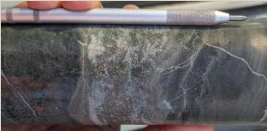
Sericite altered sandstone with quartz anhydrite pyrite vein at 1047m.
