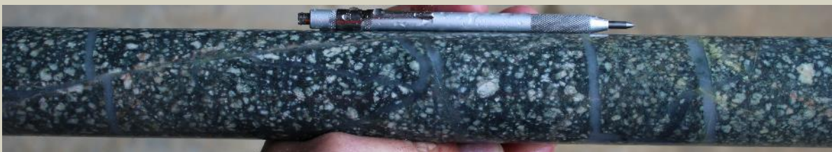
Quartz+-magnetite veining in sodic altered QDP at 1511.0m
