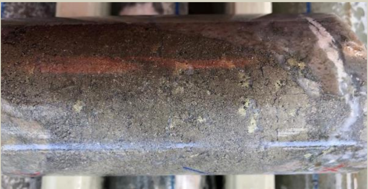
Chalcopyrite overgrowing pyrite in a D vein from 737.5m
