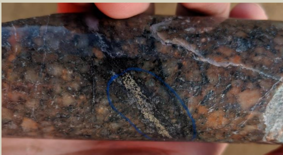
Red rock altered QDP with quartz magnetite veining hosting pyrite and chalcopryite at 1653.6m.
