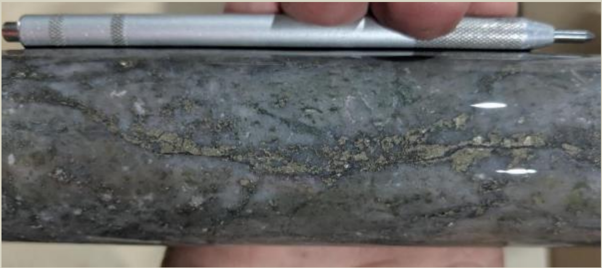
Pyrite vein in strongly sericite altered QDP. Similar in character to the NSS pyrite veining without the high sulphidation minerals at 1396.6m.
