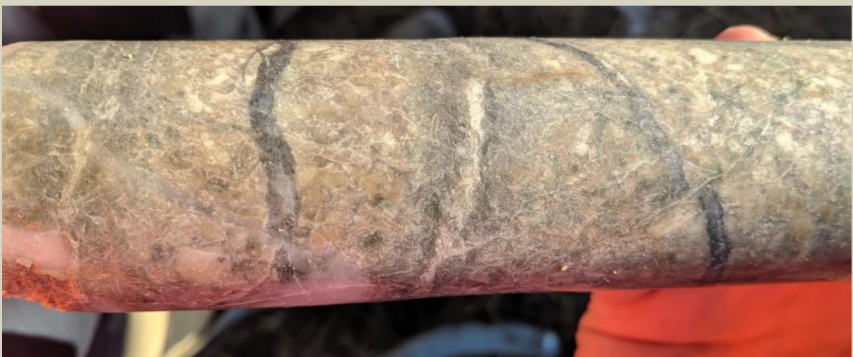
Quartz magnetite veining in a sericite altered QDP at 1623.5.
