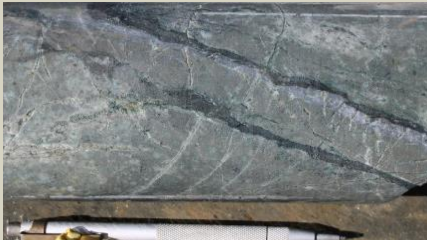
Subparallel quartz and partially demagnetised magnetite veins at 310.7m
