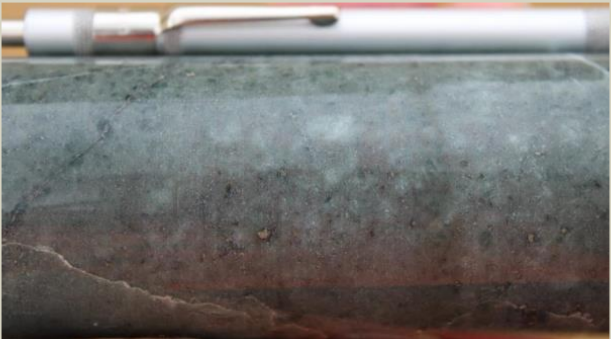
Very trace biotite alteration in quartz diorite porphyry at 1254.3m.
