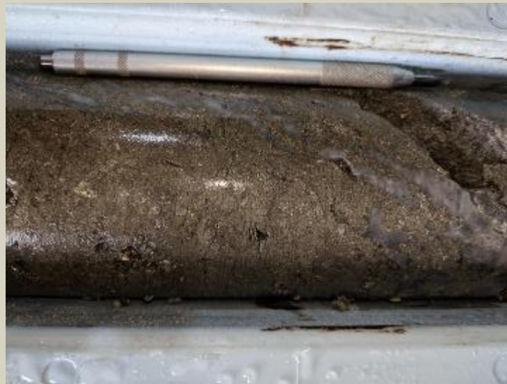
Massive pyrite D vein at 220.4m.
