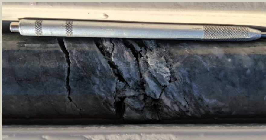
5cm wide fault zone with sericite alteration at 1673m.
