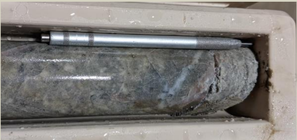
Fault gouge zone at 1423m trends steeply NNW.
