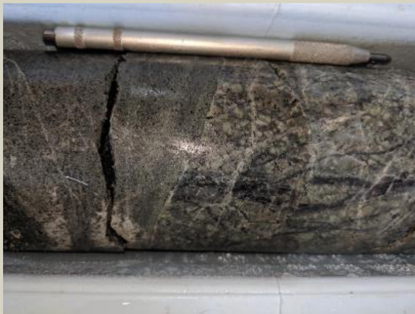
Quartz magnetite veined QDP cut by Microgabbro at 197.8m.
