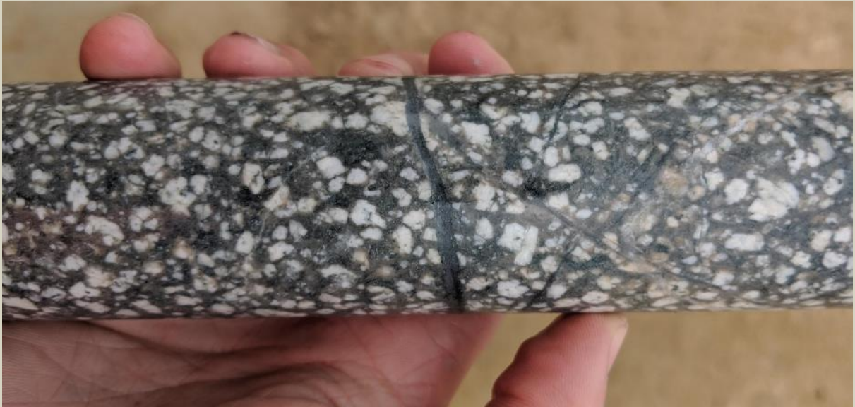
Quartz magnetite veining in an albite, actinolite magnetite altered QDP at 1692m.
