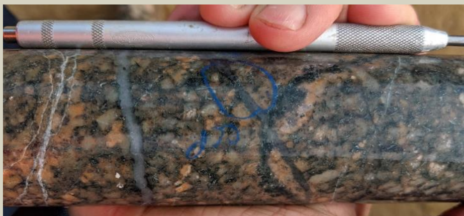
Hematite magnetite albite actinolite altered QDP with well developed M veins hosting pyrite and very trace chalcopryite at 1652.6m.
