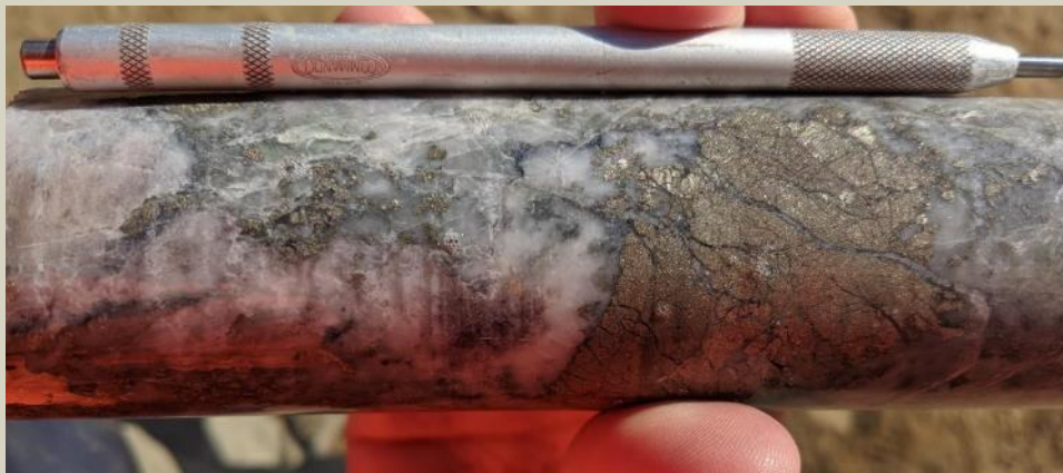
Quartz pyrite anhydrite molybdenite vein at 1622.3m.
