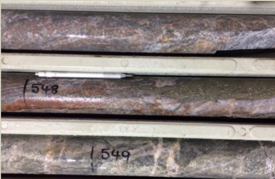
Quartz pyrite veining with later anhydrite at 548m.
