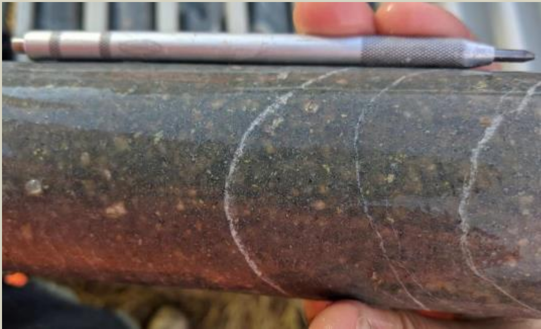
Dacite porphyry with disseminated epidote alteration and hematite dusting at 1007m.
