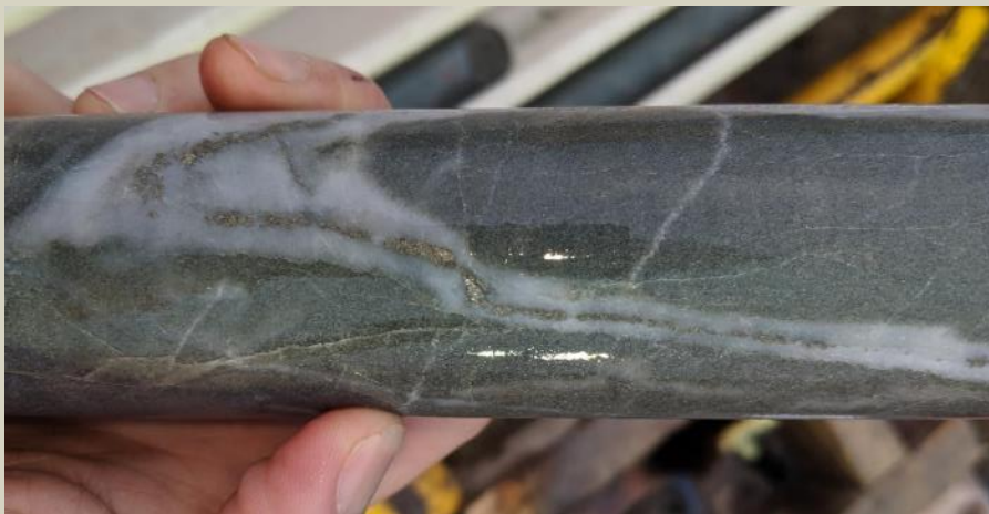
Quartz B vein with pyrite centre seam at 1560m.
