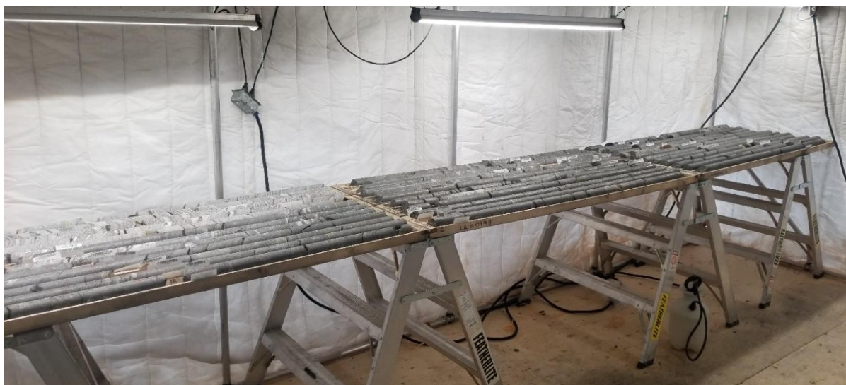
Figure 9: Drill core of DDH LR19-09 which intersected the Carheil Graphitic Trend over an extensive thickness of 70.0m
