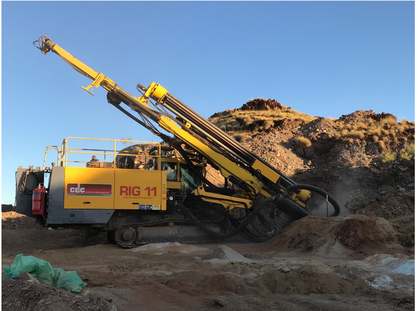
Figure Three: Castle Drilling RC rig undertaking the 12.5m x 12.5m Resource conversion programme at Klondyke, taken from the eastern side of the proposed pit looking north-west.
