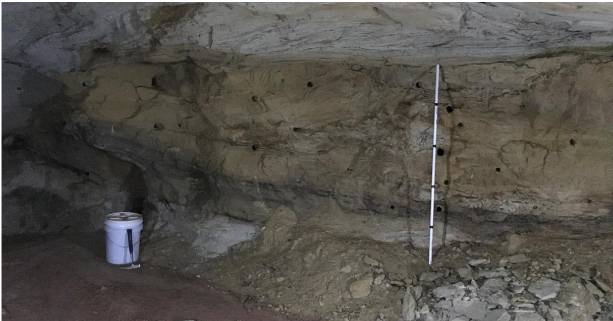
Figure 3: Thick mineralised lens exposed in the underground workings at the Jeffrey project
