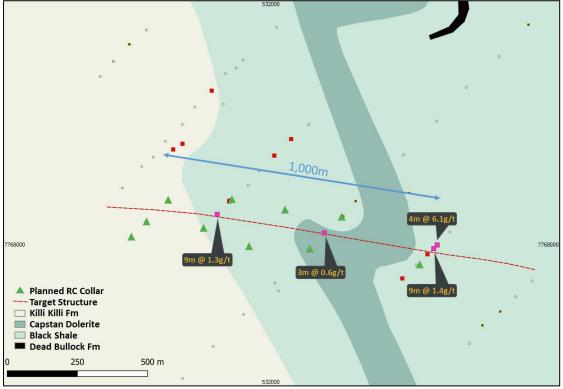
Figure 3 - Planned RC drillhole collars at the Capstan North Target with 2018 drill results
