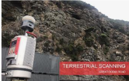
Terrestrial 3D scanning of Great Ocean Road for stability monitoring
