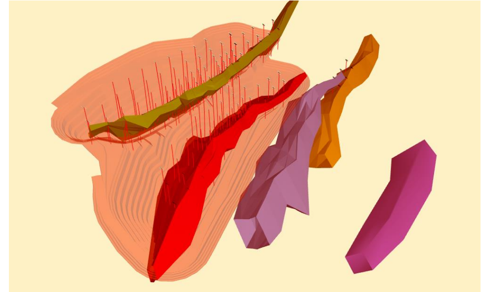
Pegmatite Dykes shown in colour against the initial open pit at Goulamina
