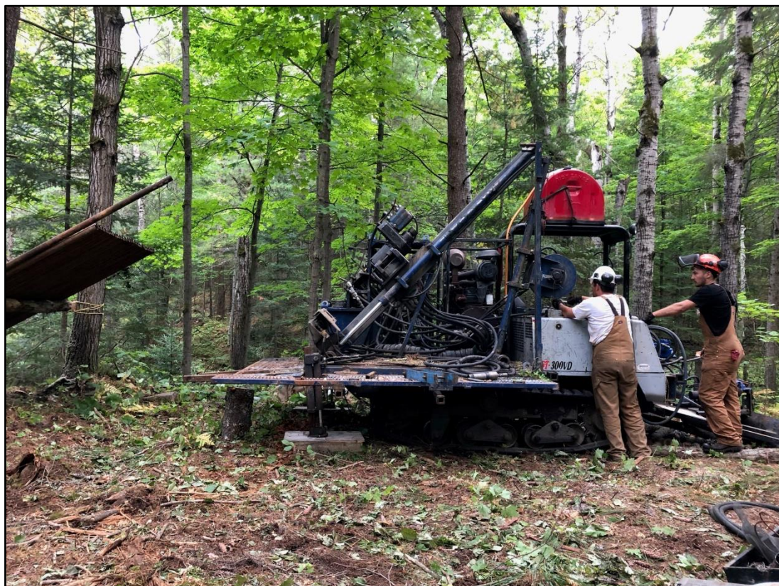
Image 1. Diamond Core Drill Rig setting up at the Panache Project
