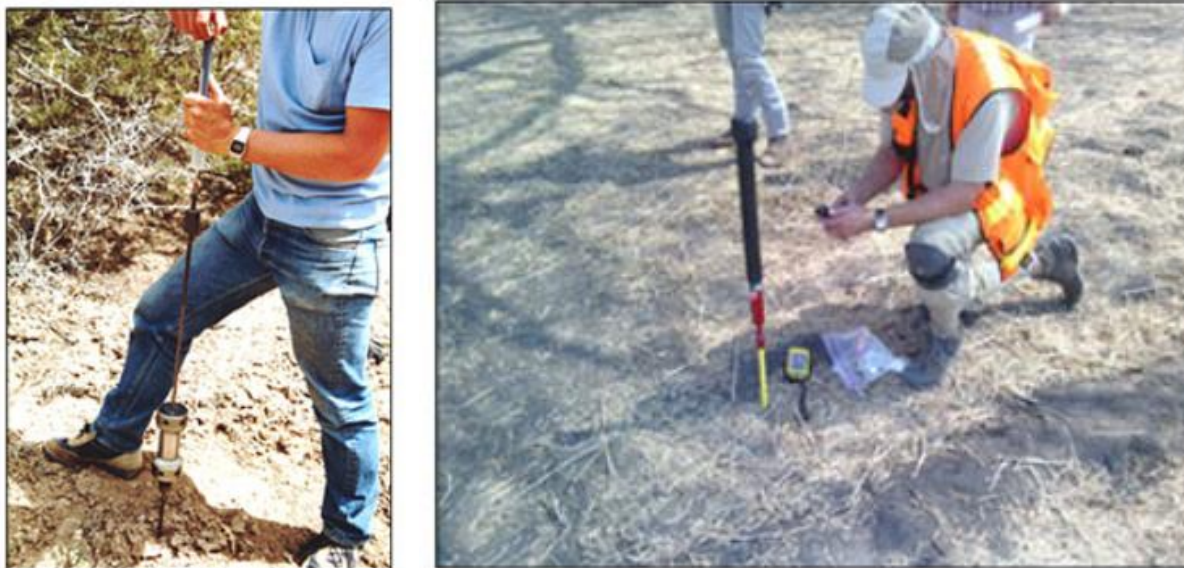
Figure 1, Specialised hand-held steel probe for sampling soil gas
