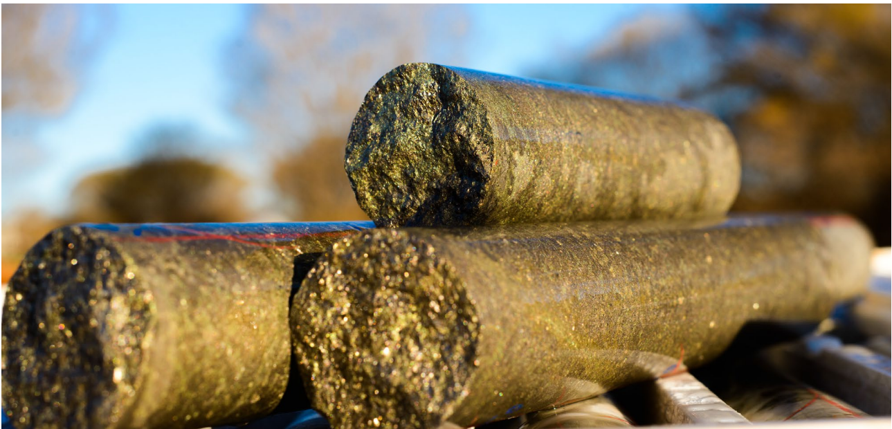
Figure 2 – drill core from the massive sulphide interval in MAD157 at 196m downhole
