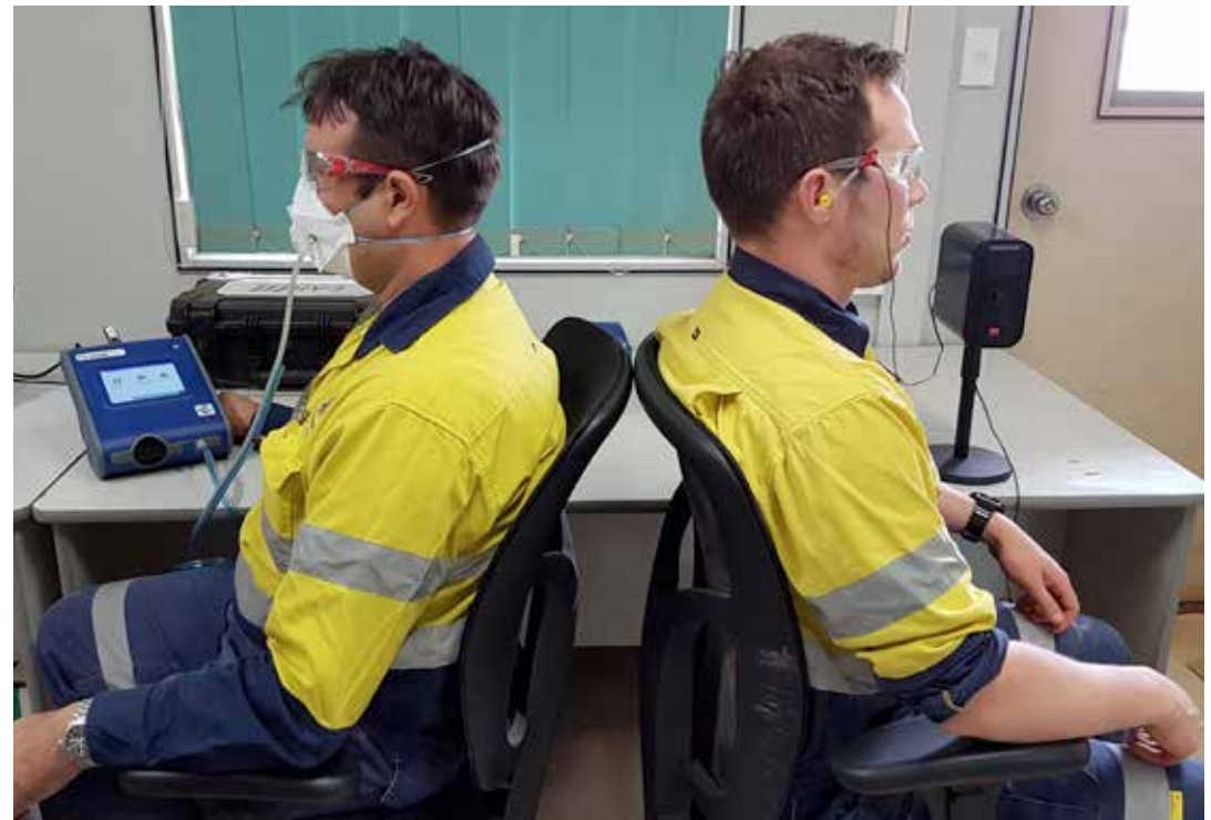
Photo: Respirator face-fit testing and E-A-RFit validation testing
