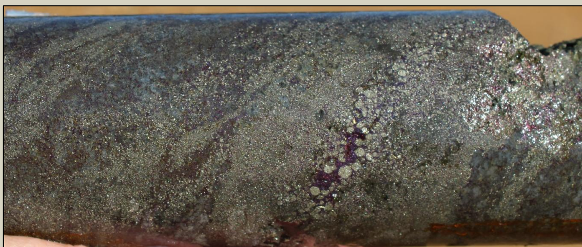
Photo 5. Quartz-pyrite-chalcopyrite-bornite veining at 150.1m in SMD051.
