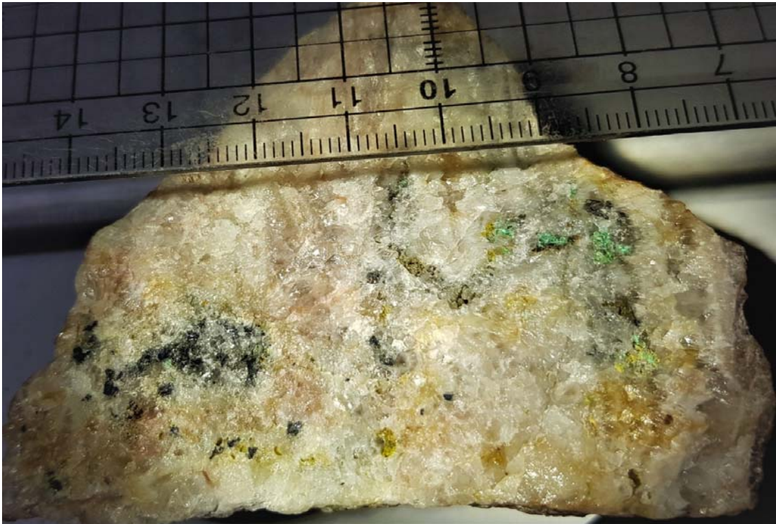
Photograph 4: Mineralised quartz from the Thumbo epithermal vein at rock chip sample site S033. This sample returned 551ppm Cu (although much of the copper was lost during sampling), over 2000ppm Pb, 0.9g/t Ag and 84ppb Au.
