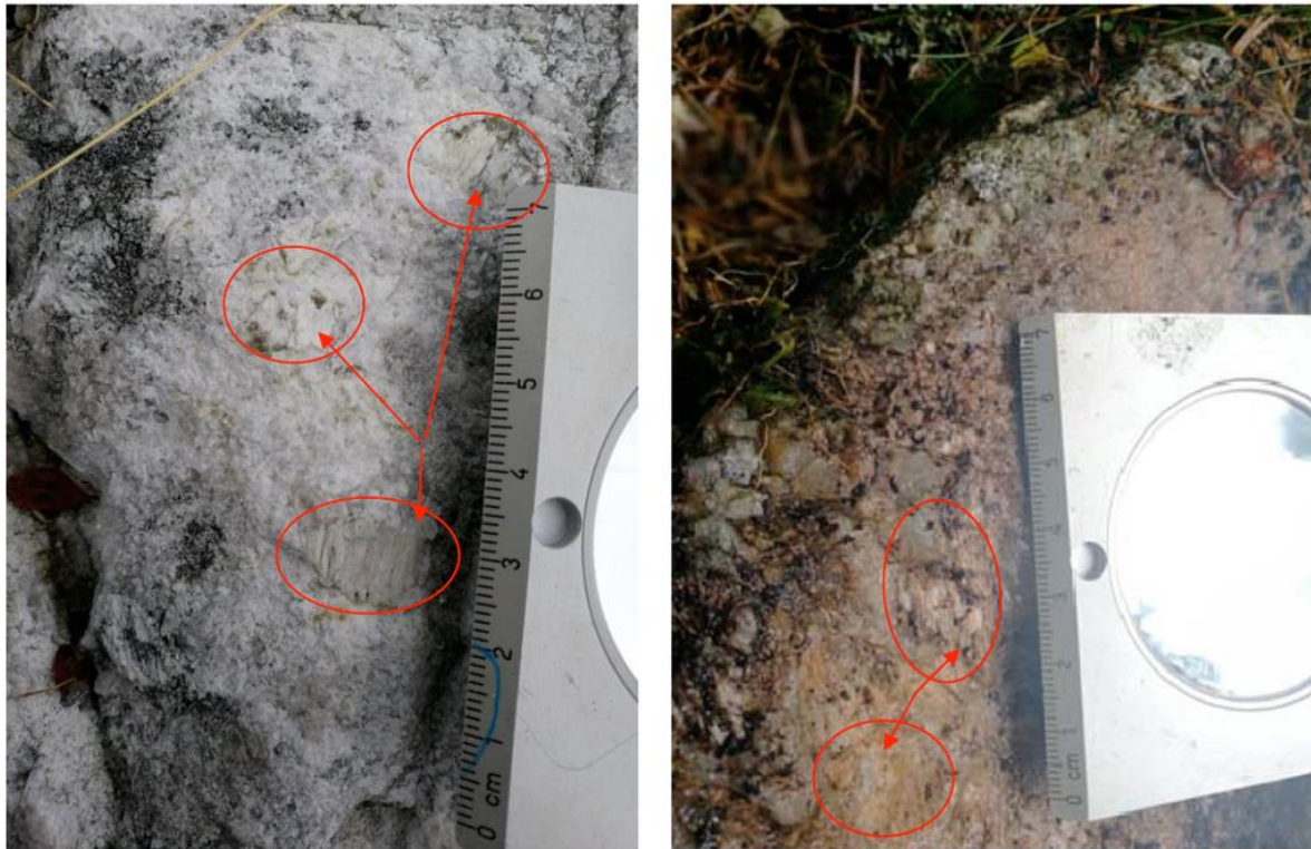
Figure 13 – Field samples with spodumene (1 cm) crystals embedded into a qtz-feldspar matrix. Figure left sample 75001 3.39% Li 2 O, Figure right sample 75010 1.68% Li 2 O.
