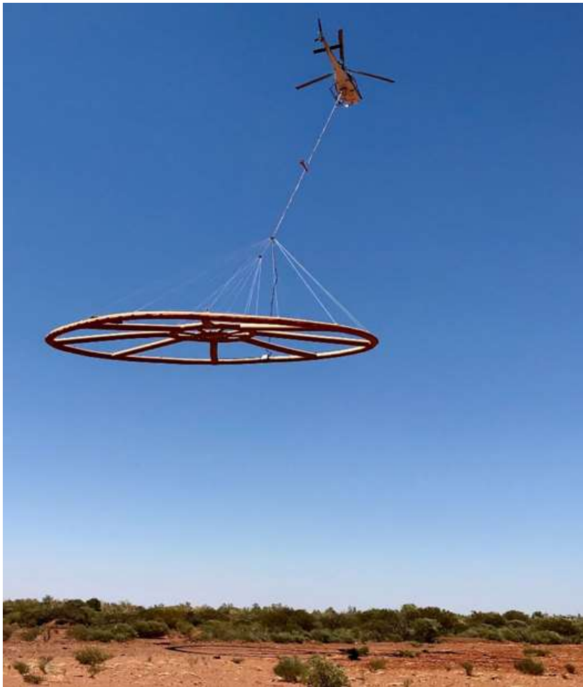
Figure 3: AEM Survey Helicopter in action
