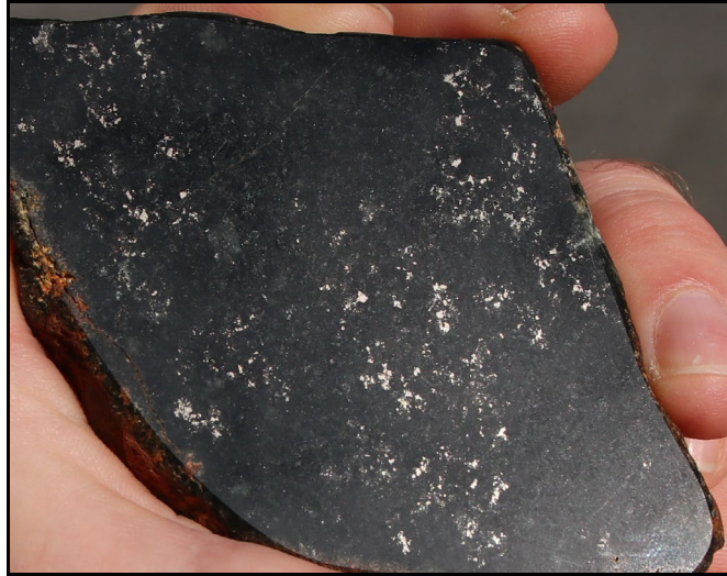
Figure 1. Quick Shears outcropping nickel-copper sulphide hand specimen
