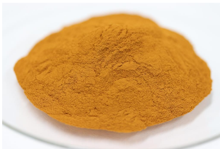
Figure 1: Photograph of High Purity 99.53% V_2O_5 Product from Gabanintha
