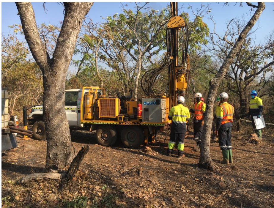
Figure 2: Canyon Resources RAB drilling rig operating at Minim Martap
