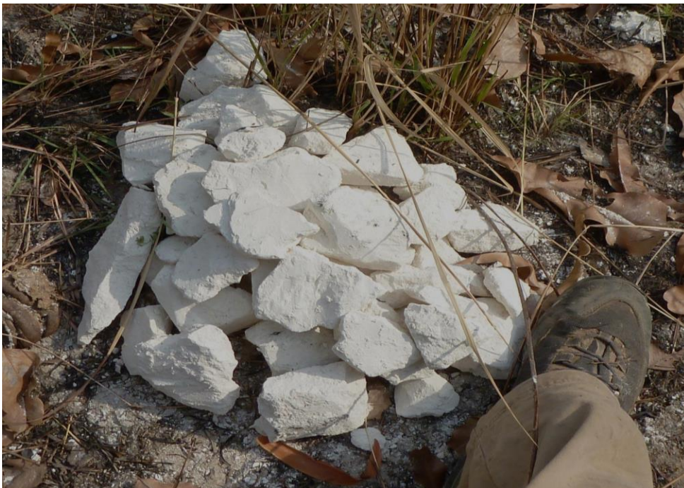
Figure 6: Fine grained, massive and brilliant white coloured Mayouom kaolin
