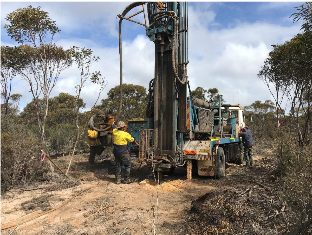
Figure 2: Challenge Drilling AC rig in action at Mount Ridley's augur gold geochemical anomaly drilling program
