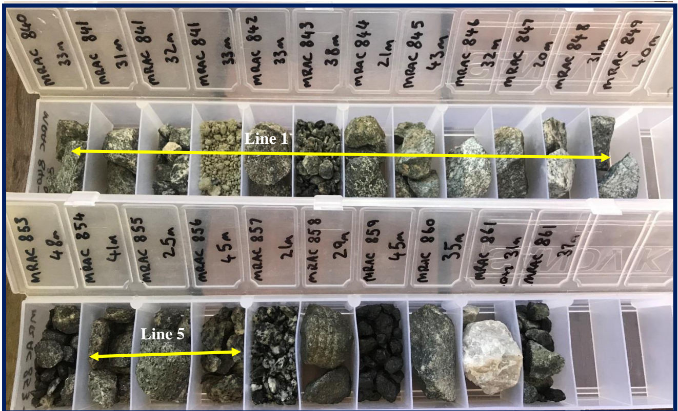
Figure 5: Chip trays from lines 1 & 5 with coarse-grained varitextured gabbronorite and olivine-bearing peridotite lithologies in end of hole samples
