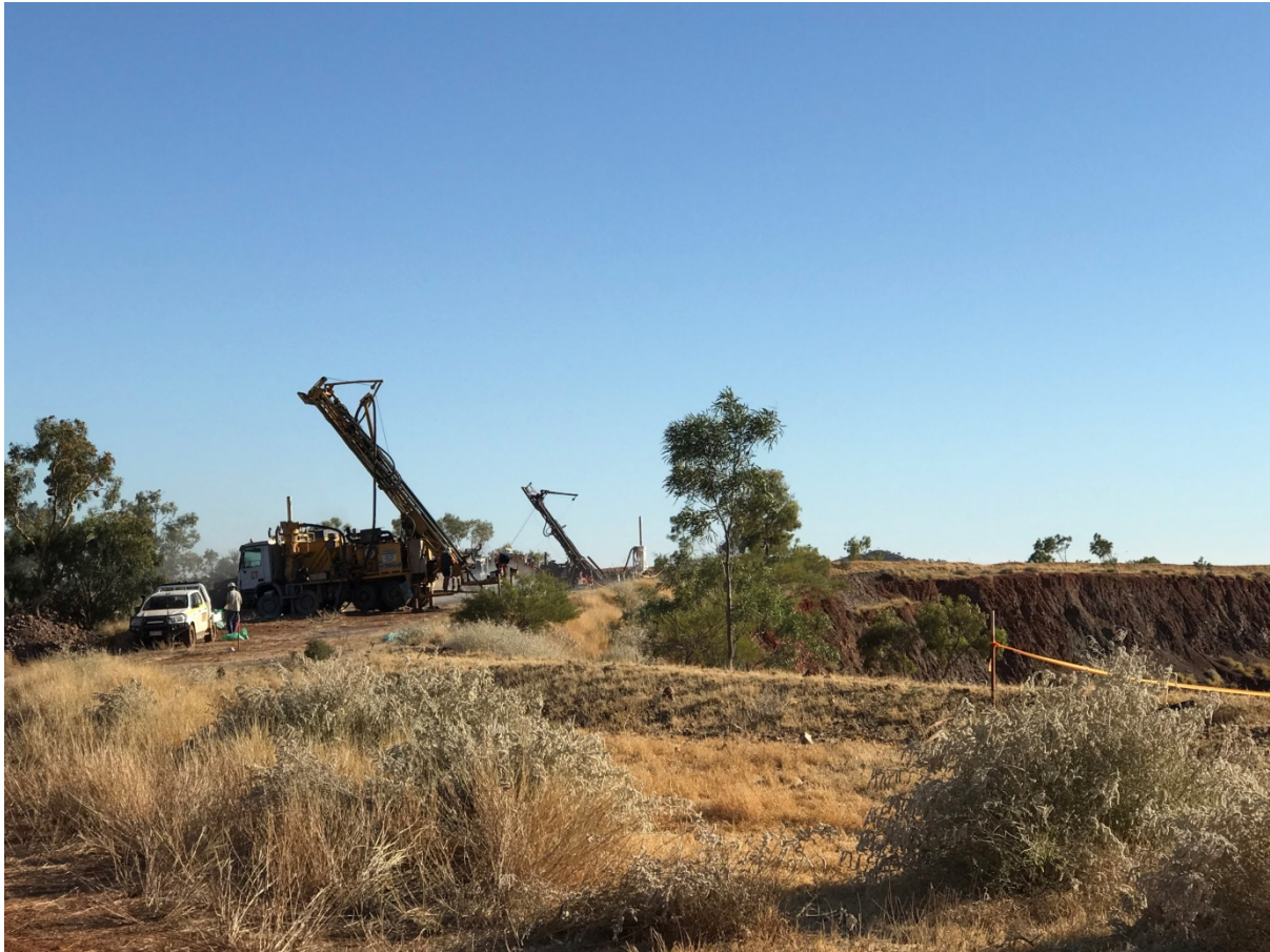
Figure 5: RC drilling beneath the Tick Hill open pit.
