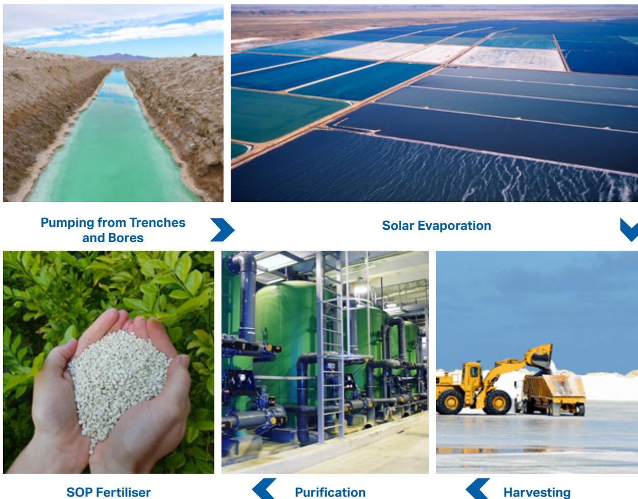
Figure 8.2: A visual representation of the production of a solar evaporation SOP project.
