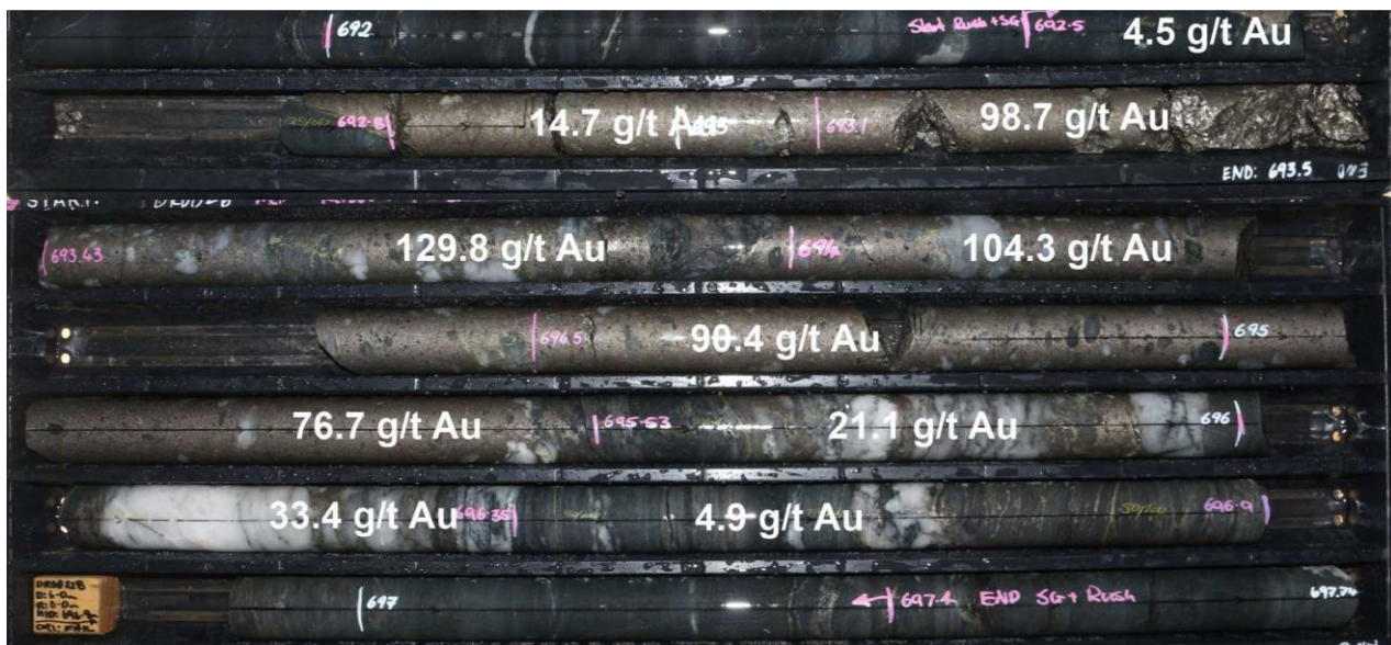
Figure 2: Deacon high grade ore shoot-massive pyrrhotite with trace chalcopyrite, quartz clasts and numerous visible gold grains in DRDD218. Interval assayed 4.4 m @ 62.4 g/t gold from 692 m. (refer asx 10/09/19)
