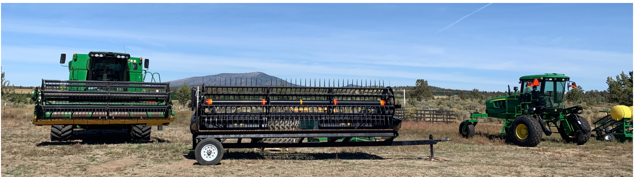
Figure 3: (Left to right) A combine harvester, swather (windrower) attachment and swather (windrower) arriving on site ahead of harvest.
