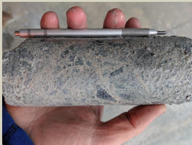
Clay altered fault breccia at serpentinite contact at 199.2m.
