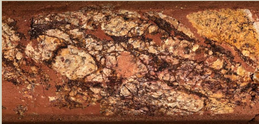
Anastomosing hematite-filled fractures after pyrite, in dacite porphyry. 9.8m
