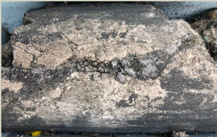
Quartz+pyrite vein in intensely clay-altered dacite porphyry. 29.3m
