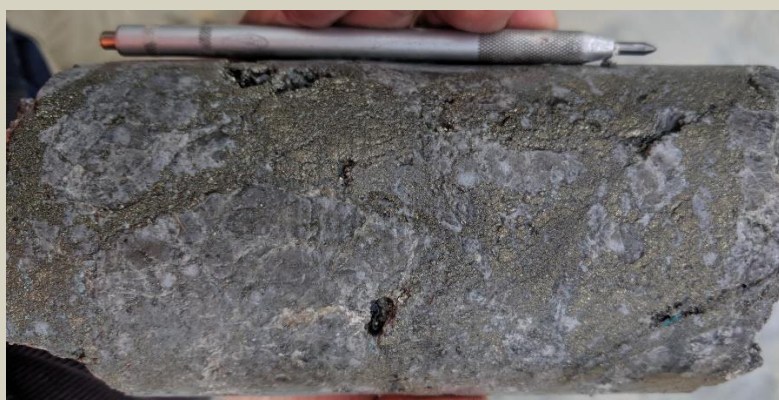
Semi massive pyrite with trace chalcopyrite and silica alteration at 78.3m.
