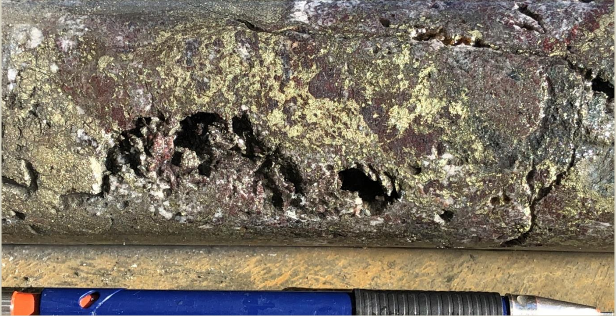
Hematite+chalcopyrite>>pyrite+quartz, vuggy semi-massive sulphide. 201.9m
