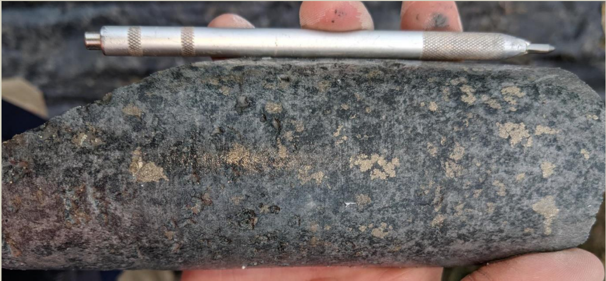
Course grained sandstone with disseminated pyrite and chalcopyrite at 111.8m.
