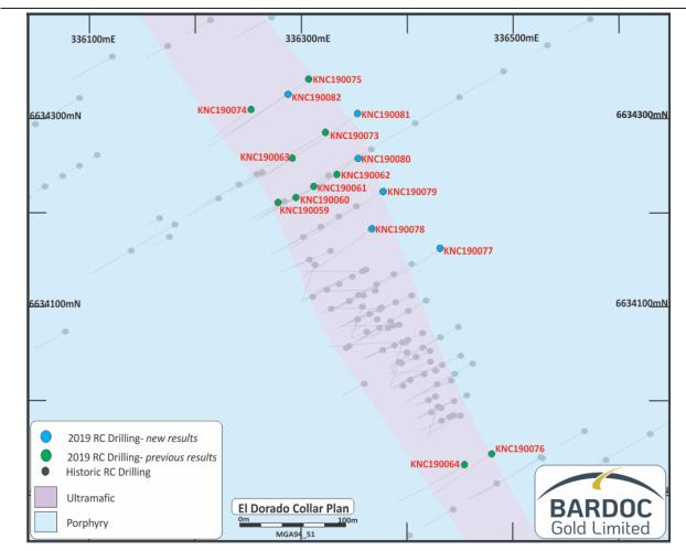
Figure 2. El Dorado drill-hole location plan
