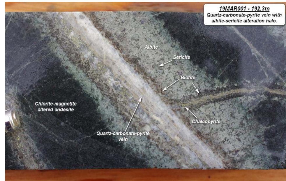
19MAR001 at 192.3m depth. Quartz-carbonate-pyrite-chalcopyrite veins with biotite and feldspathic/sericitic haloes. Likely to be multiphase.
