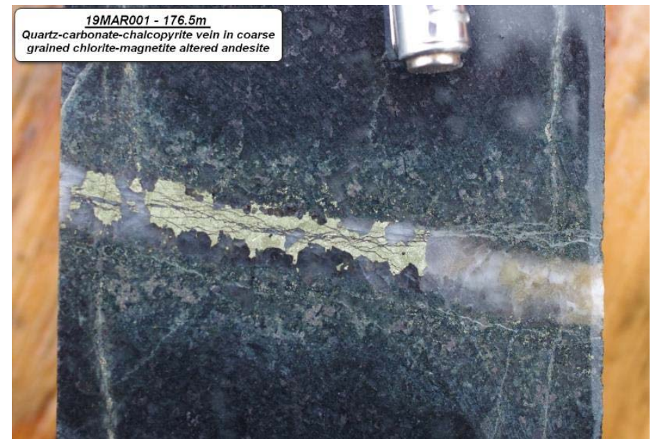
19MAR001 at 176.5m depth. Quartz-carbonate-chalcopyrite vein with weak selvage of chlorite and sericite(?).
