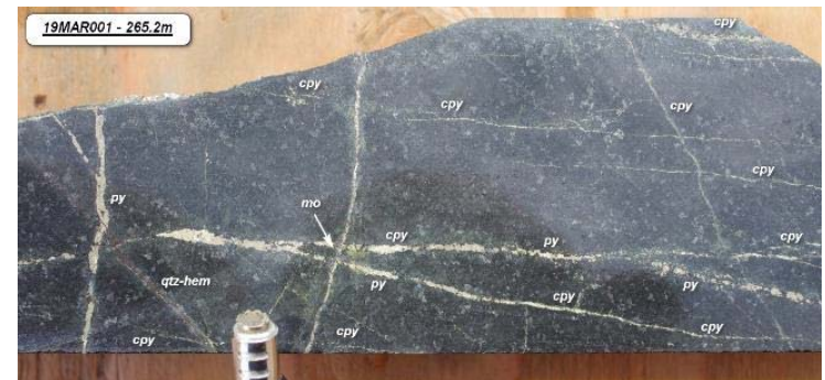
19MAR001 at 265.2m depth. Pyrite and chalcopyrite vein networks overprinting sericite-chlorite-magnetite altered andesite.
