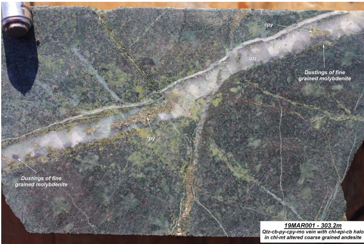
19MAR001 at 303.2m depth. Quartz-carbonate-pyrite-chalcopyrite-molybdenite vein cutting epidote chlorite-magnetite altered andesite.
