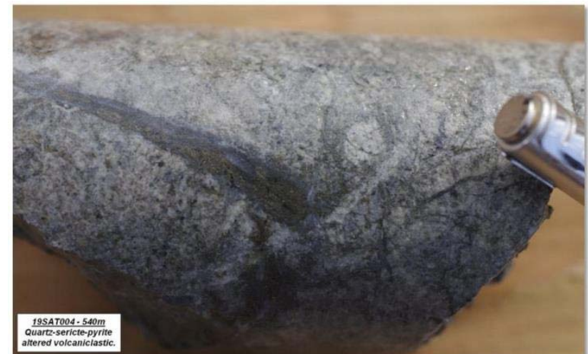
19SAT004 at 540m depth. Quartz-sericite-pyrite veining and alteration overprinting andesitic volcanic rocks.
