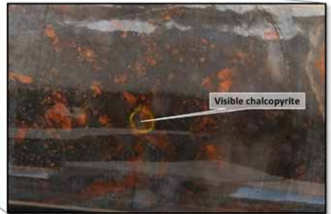
Figure 5: Close up of a zone of intensely altered, red oxidized granitic dykes and grey quartz veins. Chalcopyrite is located in the quartz adjacent to the red dyke fragments.
