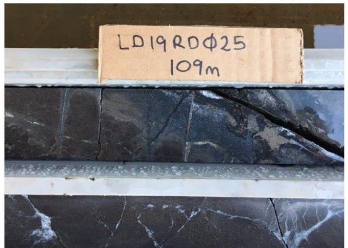
Image 3. Diamond Core photos LD19RC025 with IOCG style sulphide mineralisation (95– 109 m)
