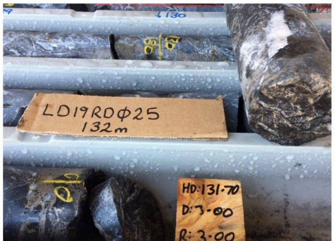
Image 4. Diamond Core photos LD19RC025 with IOCG style sulphide mineralisation (112– 132 m)
