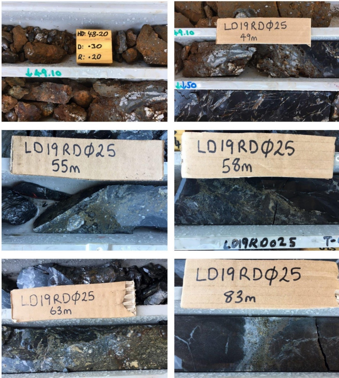
Image 2. Diamond Core photos LD19RC025 with IOCG style sulphide mineralisation (48 – 83 m)
