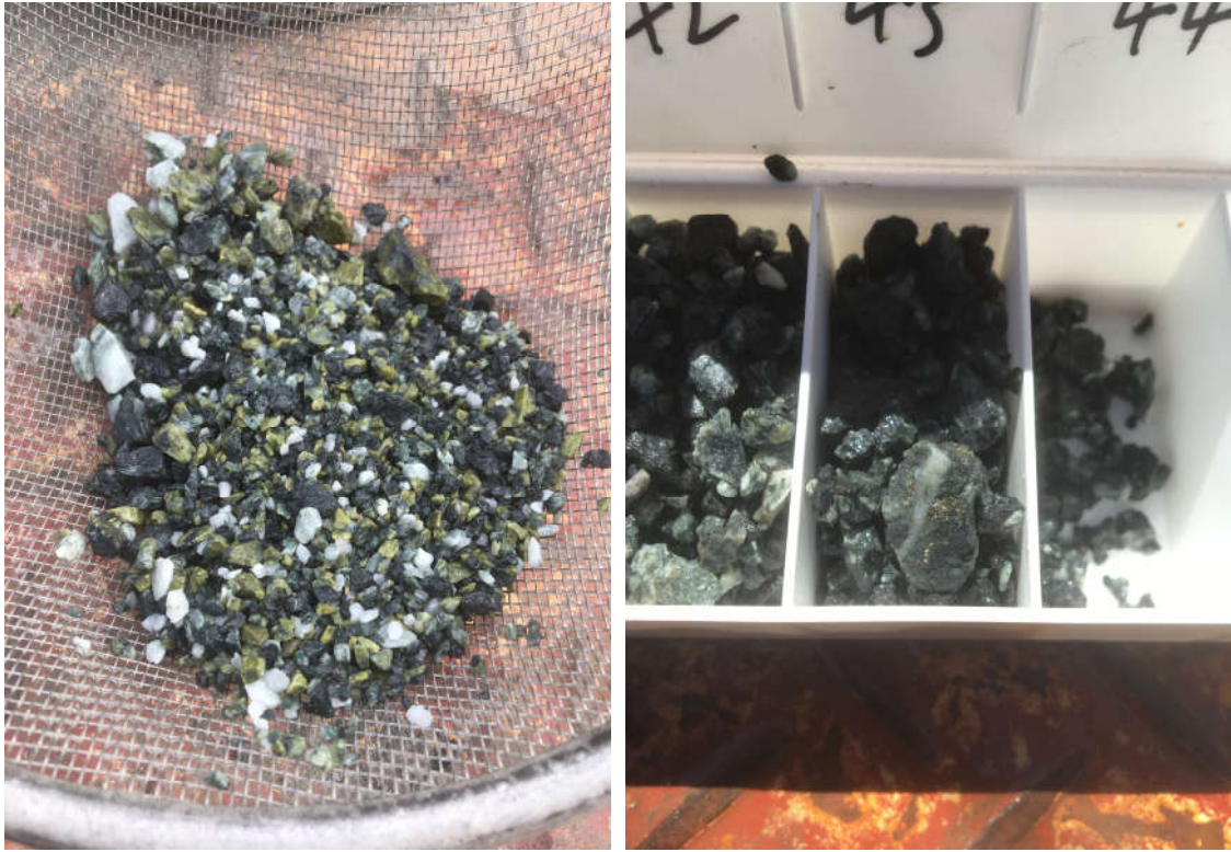
Figure 2: Victory Bore rock chips displaying alteration, veining, and mineralisation
