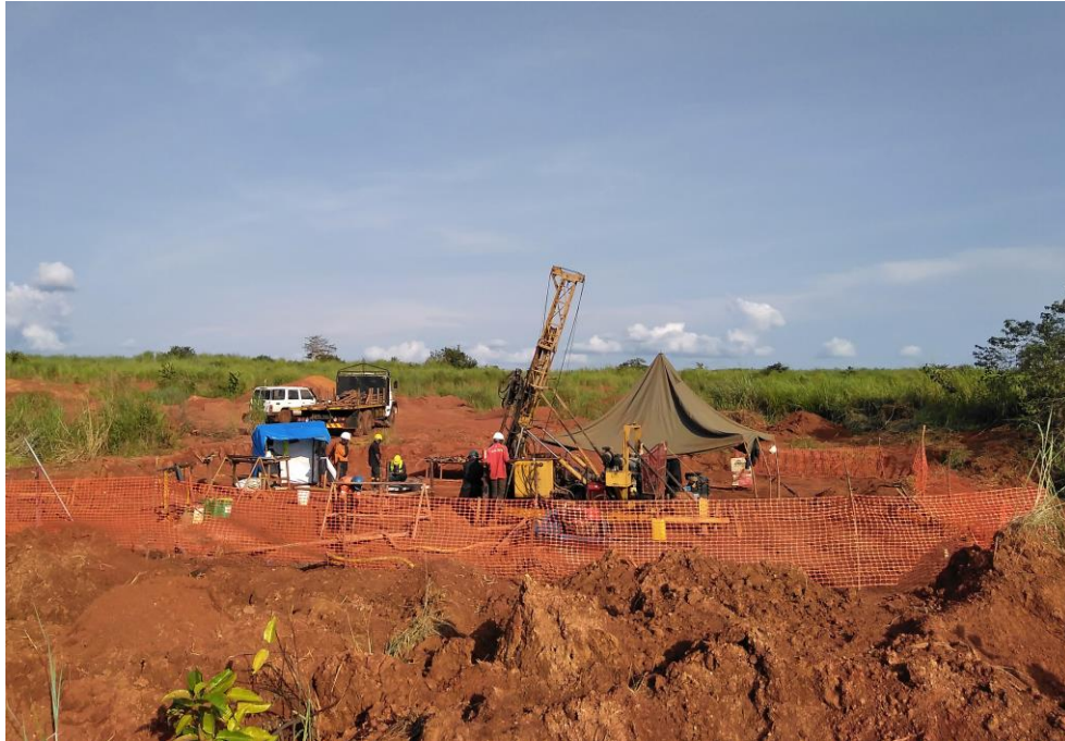
Photograph 1. Diamond core drill rig in operation at drillhole GRDD035
