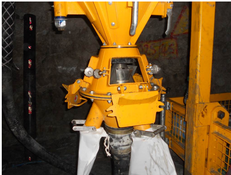
Figure 3 - The rotary splitter and sample bags
