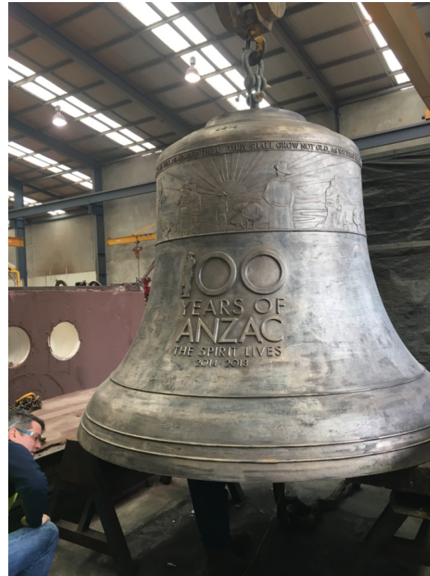
VEEM recently cast the biggest swinging bell in the southern hemisphere – 6.5 tonnes.
